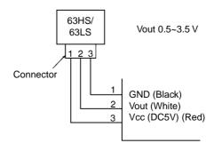
\*Connector connection specifications on the pressure sensor body side.
