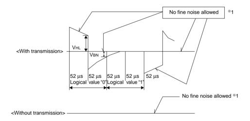
Check the wave shape of transmission line with an oscilloscope to confirm that the following conditions are being satisfied.
