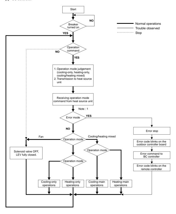
Note: 1 Two error modes include indoor unit side trouble, BC controller trouble, and heat source unit side trouble. In the case of indoor unit side trouble, error stop is observed in the concerned indoor unit only, and in the cases of BC controller and heat source unit side troubles, error stop is observed in all the indoor units, BC controller, and heat source unit.
