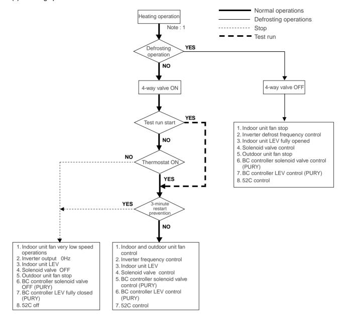
Note: 1 When outdoor unit starts defrosting, it transmits defrost operations command to (BC controller and) indoor unit, and the indoor unit starts defrosting operations.
