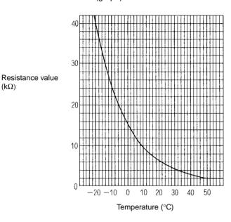
$$\label{eq:Resolvent} \begin{split} & \text{Thermistor R}_0 \!\!=\!\! 15 \ k\Omega \\ & \text{Rt} \!\!=\!\! 15 \text{exp } 3460 \ \left\{\!\! \left( \frac{1}{273 \!\!+\!\! t} \!-\! \frac{1}{273t} \right) \!\! \right\} \end{split}$$
