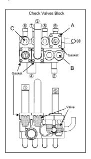
\* Closed torque: A: 1.7kg·m (0.17N·m)
