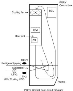
PQRY Control Box Layout Diagram (Internal air passages)
