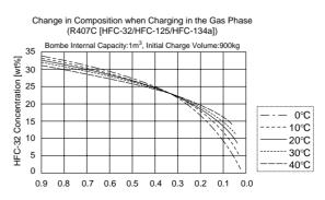
Proportion Remaining in Bombe (Volume Remaining in Bombe/Bombe Internal Capacity) [kg/  $\ell$ ]
