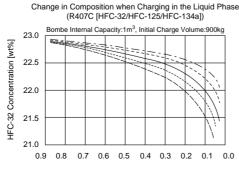
Proportion Remaining in Bombe (Volume Remaining in Bombe/Bombe Internal Capacity) [kg/  $\ell$ ]
