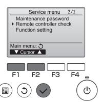
② Select "Remote controller check" from the Service menu, and press the button to start the remote controller check and see the check results.
