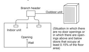
(c) If the smallest room has mechanical ventilation apparatus that is linked to a household gas detection and alarm device, the calculations should be performed for the second smallest room.
