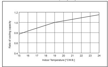
Figure 8 Outdoor unit temperature correction To be used to correct outdoor unit capacity only
