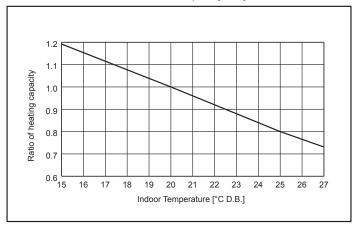
Figure 10 Outdoor unit temperature correction
