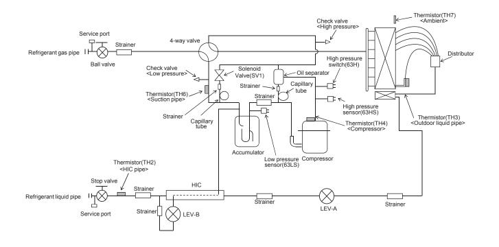
Capillary tube for oil separator :  $\phi$ 2.5× $\phi$ 0.8×L800 Capillary tube for solenoid valve :  $\phi$ 4.0× $\phi$ 3.0×L500
