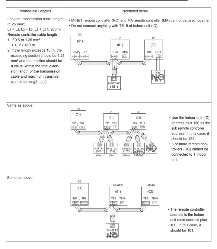
B. Example of a group operation system with 2 or more outdoor units and a M-NET remote controller. (Address settings are necessary.)
