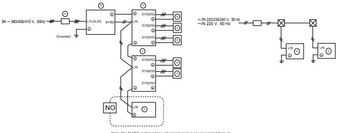
Note: The M-NET control indoor unit cannot receive power supplied from an outdoor unit, so provide it with power separately.
