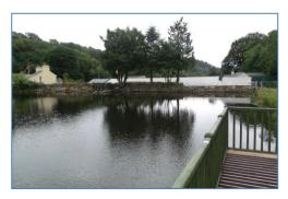
ABOVE: The Salmon Lake is used to help dissipate heat, whatever the season using an open-water, slinky-based system.
