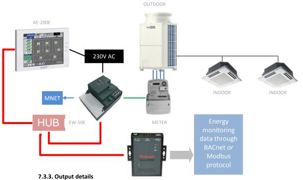
The energy monitoring data is calculated by the AE-200E and EW-50E and is available on BACnet or Modbus.
