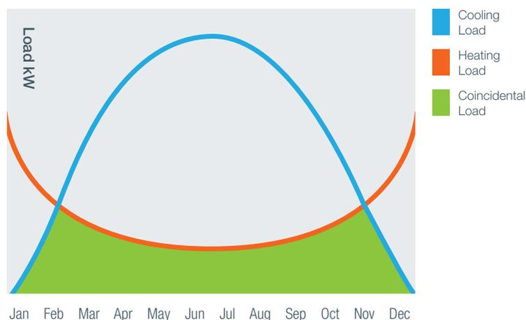
Chillers that are able to provide simultaneous heating and cooling during these periods of coincidental load, provide significant reductions in energy usage and running costs.
