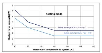
Minimum water content: in the case of i-BX-N units (heat pump, reversible), the highest value between refrigeration and heating operation must be considered. Use water / glycol mixture for water temperature below + 5°C.
