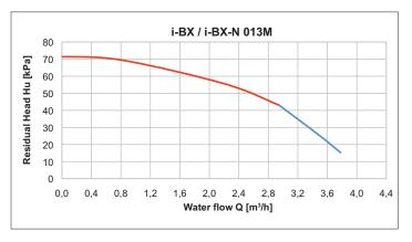
The pressure head values refer to the pressure available at the connections to the unit.
