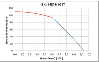
The pressure head values refer to the pressure available at the connections to the unit.
