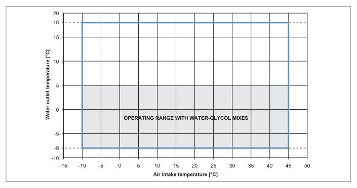
Operation in cooling mode: System circuit temperature difference, minimum 3°K, maximum 8°K Maximum glycol content 40%
