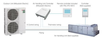
One air handling unit controller is required per heat exchanger If using more than one air handling unit controller on a single AHU, there are two options:
