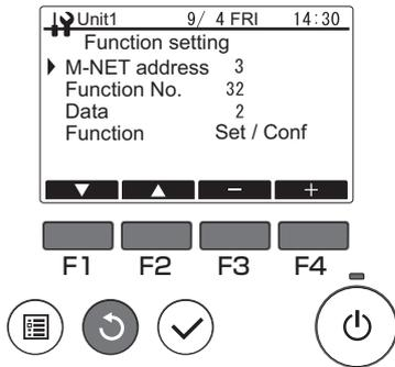
Once data transmission is completed, the screen indicating that the settings have been made will be displayed. To continue making settings, press the [Return] button to return to the screen in procedure 3. Use the same procedure to set other connected unit and Data settings.
