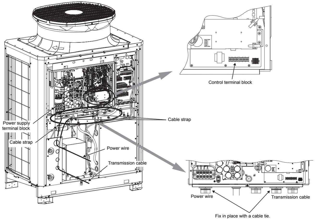
**Important:** Power supply cables larger than 25 mm<sup>2</sup> in diameter are not connectable to the power supply terminal block (TB2). Use a pull box to connect them.
