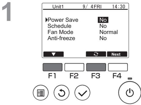
In the Operation setting screen, press the [F1] button to move the cursor to Power Save.
