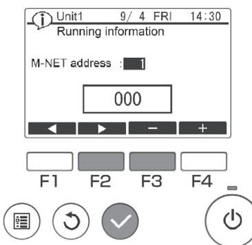
Set the desired M-NET address with the [F2] and [F3] buttons, and press the [Select] button.
