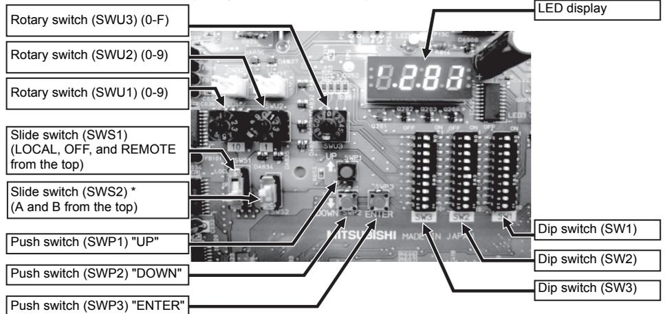
Set the slide switch SWS2 on the board inside the control box to the **lower side** during the trial run.
