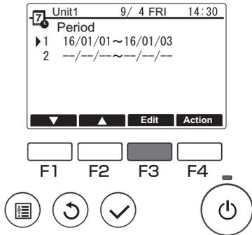
Press the [F3] button to proceed to the settings screen. You can set 2 types of pattern, as necessary.
