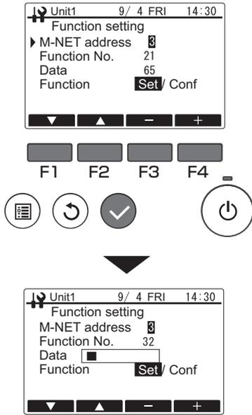
The Function setting screen will be displayed. Press the [F1] or [F2] button to select the connected unit "M-NET address", "Function No." or "Data", and then press the [F3] or [F4] button to change to the desired setting. After changing to the desired setting, press the [Select] button. The setting data transmission screen will be displayed.
