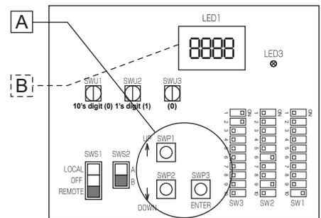
Following the steps above, set the value for the following items with the switches on the circuit as necessary. Item [106] must be set when multiple units are connected to a system.
