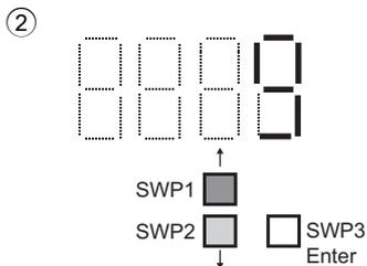
The left figure shows a display example (Code 9 Outlet hot water temperature setting).
