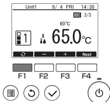
Press the [F1] button to go through the operation modes in the order of "Mode1, Mode2, and Mode3."
