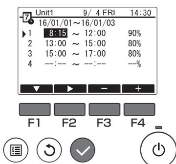
Press the [F1] to [F4] buttons to set the Power Save start time, end time and control value.
