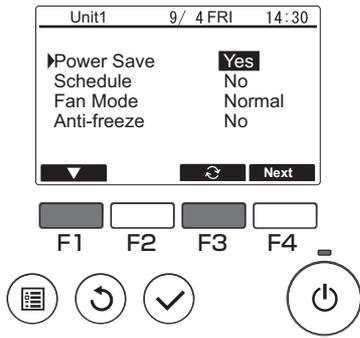
In the Operation setting screen, press the [F1] button to move the cursor to Power Save.
