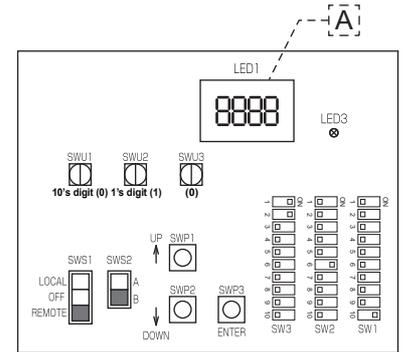
**3. Set the preset values with the switches on the circuit board.**
