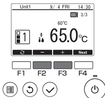
Press the [F2] button to decrease the set temperature, and press the [F3] button to increase.
