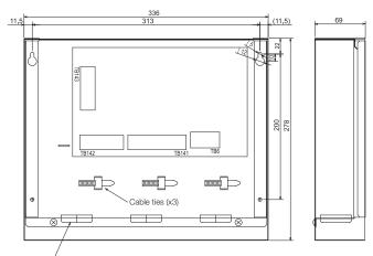
Electrical wires openings (x3). When the unit is installed these are facing down.
