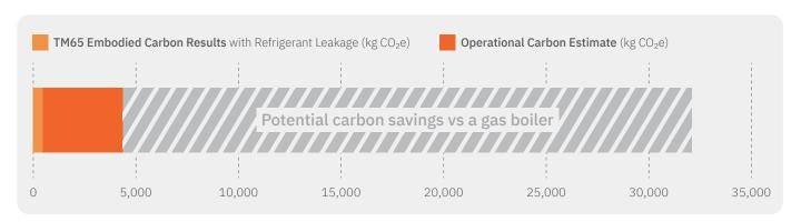
Operational carbon data for heating requirements, according to heat pump ErP fiche at medium temperature (55°C), average climate conditions and equivalent boiler heat output. (Does not include thermal store data). Gas boiler assumptions: embodied carbon of 300kg CO<sub>2</sub>e, efficiency of 93%, service life of 15 years.
