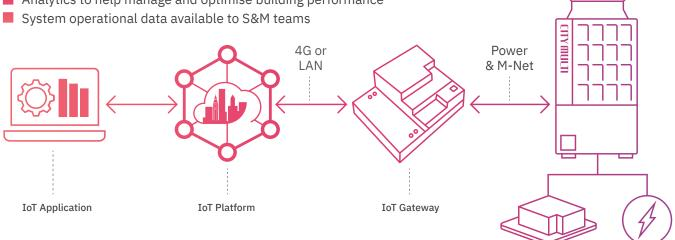
All equipment is on M-Net (network), when no central controller is present M-NET required.
