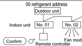
\* When grouping different refrigerant systems, if an indoor unit other than the one to which the refrigerant address has been set performs fan operation, there may be another refrigerant address that is the same as the specified one. In this case, check the DIP switch of the outdoor unit to see whether such a refrigerant address exists.
