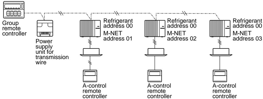
It would be ok if M-NET wire (non-polar, 2-cores) is arranged in addition to the wiring for A-control.
