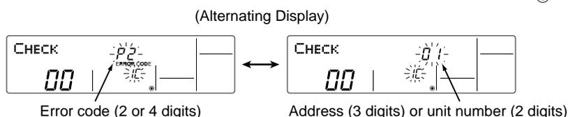
When using remote-/local-controller combined operation, cancel the error code after turning off remote operation. During central control by a MELANS controller, cancel the error code by pressing the **ON/OFF** button.
