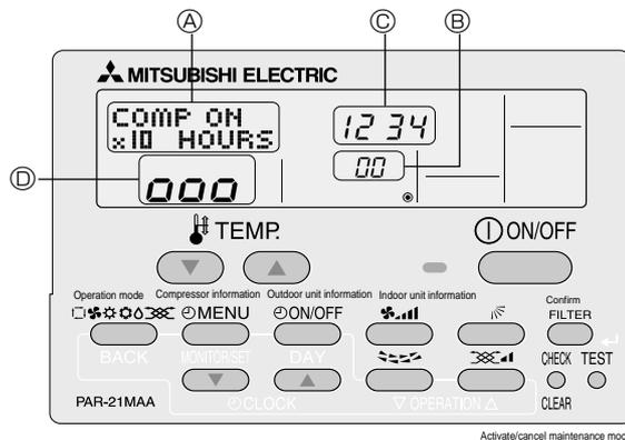
(1) Press the **TEST** button for 3 seconds to switch to maintenance mode.
