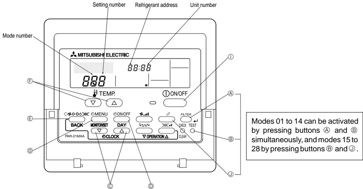
The flow of the function selection procedure is shown below. This example shows how to use the remote controller's internal sensor. (Mode No. 2: setting No. 3)
