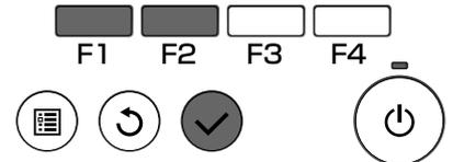
② With the **F1** or **F2** button, enter the refrigerant address, and press the
