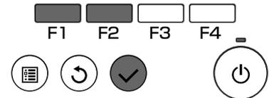
② Select "Test run" with the **F1** or **F2** button, and press the button.
