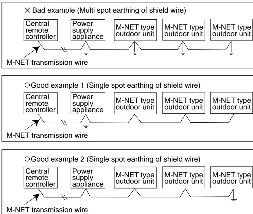
If there are more than 2 grounding spots on the shield wire, noise may enter into the shield wire because the earth wire and shield wire form 1 circuit and the electric potential difference occurs due to the impedance difference among earthing spots. In case of single spot grounding, noise does not enter into the shield wire because the earth wire and shield wire do not form 1 circuit.
