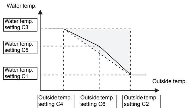
\* Always use a value for setting C6 that is between setting value C2 and setting value C4, and for setting C5 between setting value C1 and setting value C3.
