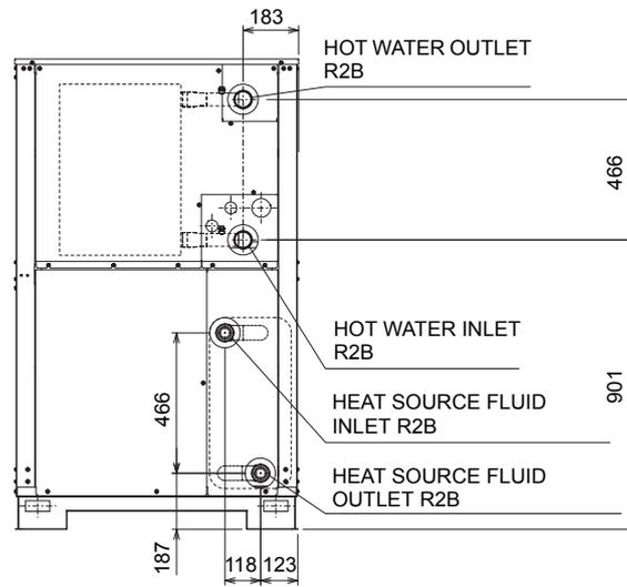
Heat source side pipe connection is normal condition.
