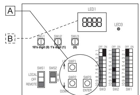
Following the steps above, set the value for the following items with the switches on the MAIN circuit as necessary. Item [107] must be set when multiple units are connected to a system.
