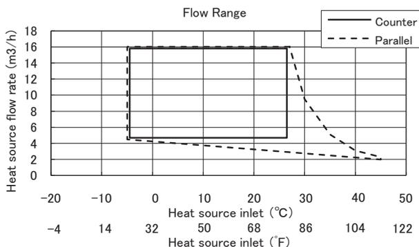
When using brine as heat source fluid
