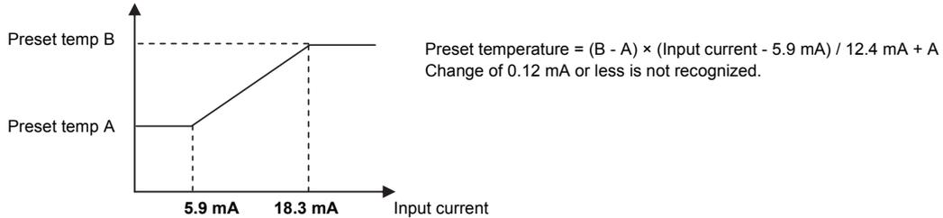
\* Due to the resistance of the wire that is connected to the 4-20 mA analog input, the preset temperature may not properly be sent. If this is the case, check the current value of the analog input, and adjust the output current value of the connected 4-20 mA signal output device.
