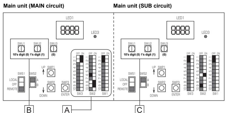
Make sure the address of the MAIN circuit on the main unit is set to "1" (labeled B in the figure above) and that the address of the SUB circuit on the main unit is set to "51" (labeled C in the figure above).
