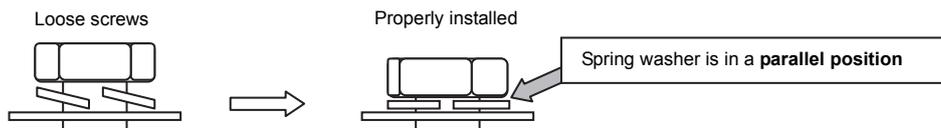
2. Check that the wiring does not move at the screw terminal.
