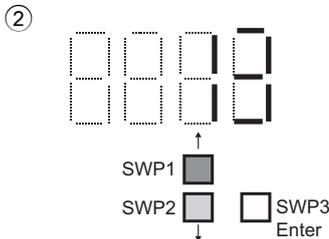
The left figure shows a display example (Code 13 Built-in thermistor temperature setting 2).
