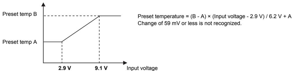
**(9) Setting the capacity control ratio using analog signal input**
