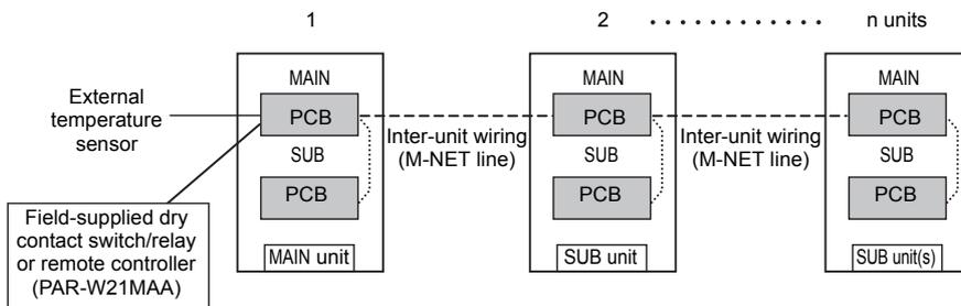
Refer to the sections "Switch Types and the Factory Settings" on the next page and "System configuration procedures: Multiple system" (page 22) for further details.
