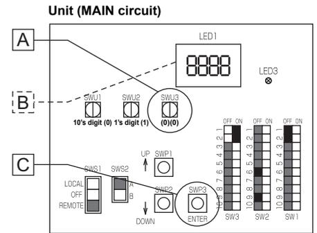
\*1 If the start-up process has already been completed, [FFFF] (instead of [EEEE]) will appear when the rotary switch SWU3 is set to "F."
