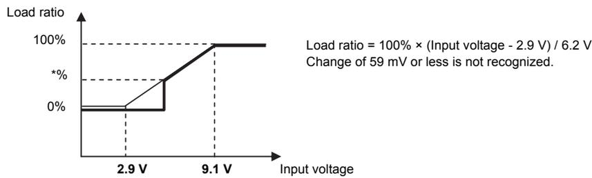
\*%: When the compressor frequency drops below 30 Hz, the compressor stops.
