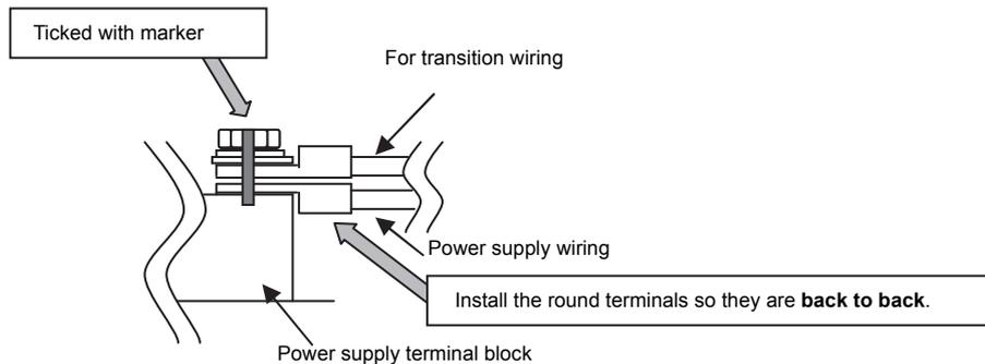
**Important:** Power supply cables larger than 25 mm<sup>2</sup> in diameter are not connectable to the power supply terminal block (TB2). Use a pull box to connect them.
