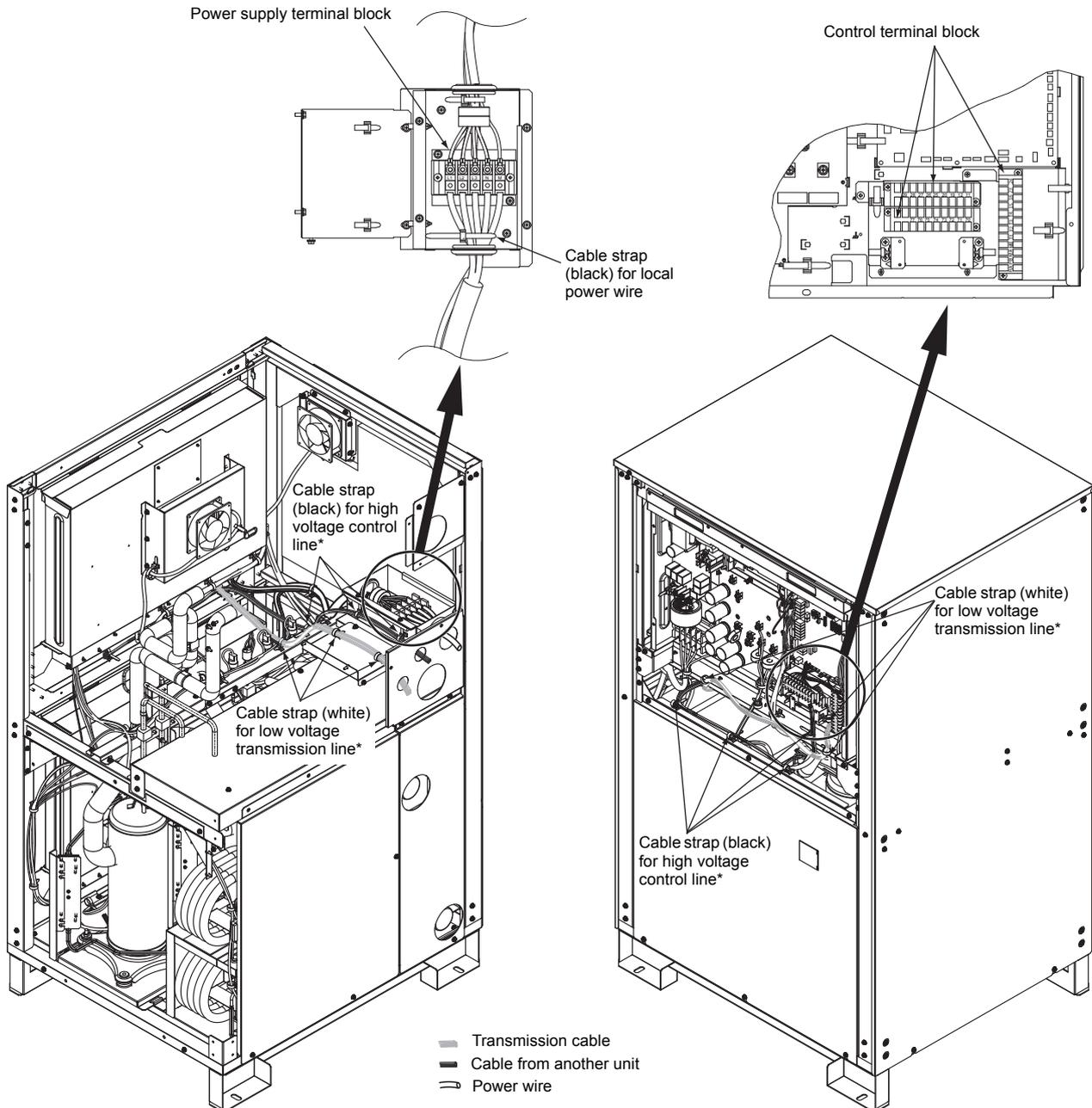
\* When connecting the cables, first temporarily fasten the cables, and then fasten them properly after the cables have been connected to the terminal blocks within the control box.
