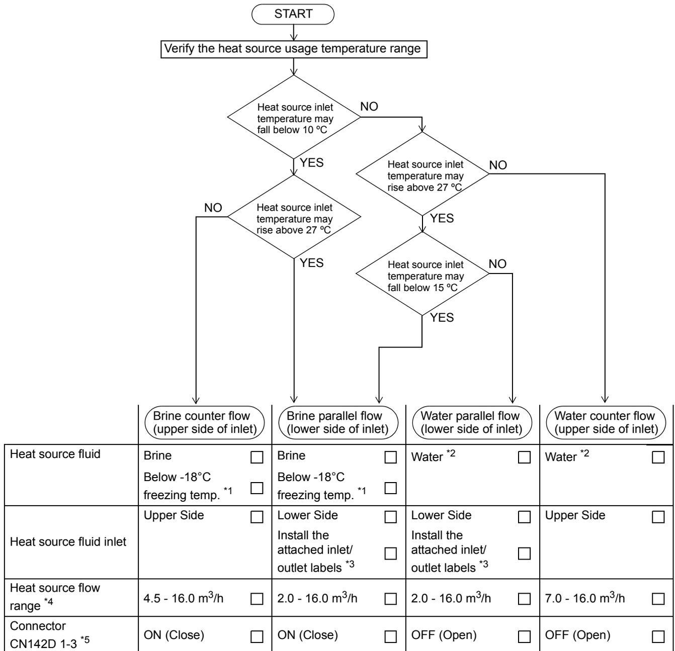
\*1 To prevent the heat exchanger from freezing, check that the concentration of brine is such that the freezing temperature is -18°C or less before operation.
