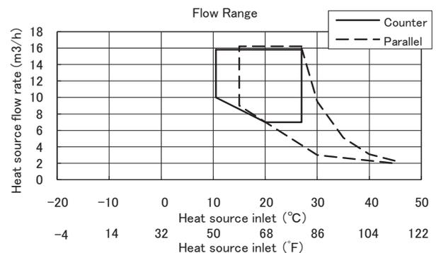
When using water as heat source fluid
