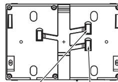
External input adapter cable access hole
