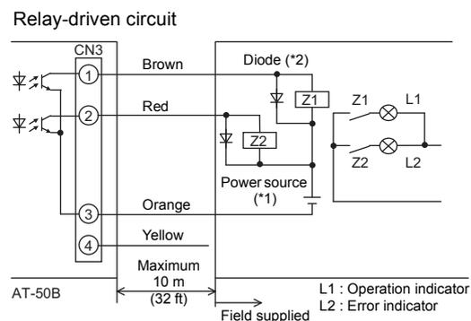
Use relays that meet the following specifications for relays indicated as Z1 and Z2 in the figure.
