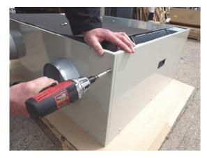
Place the top cover  $\bigcirc$  over the housing panels 7 and fix using 8 x M4 X 16 set screws (12) and 8 x nylon washers (10)
