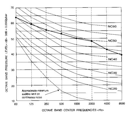
Note: The measuring point is 1m from the bottom of the unit (1m from the front of the unit)
