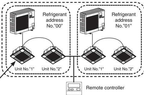
As for this air conditioner, air conditioner No. is "Unit No. 1" of refrigerant address "0".
