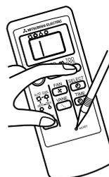
Press OPERATE/STOP (ON/OFF) button of the remote controller (the set temperature is displayed) with the remote controller headed towards the indoor unit. ※1
