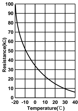
Gas pipe temperature thermistor (RT65,66)
