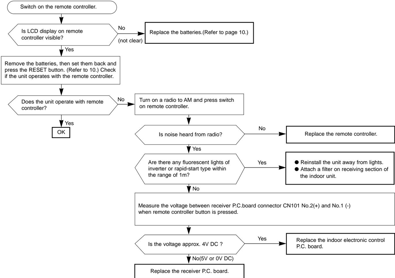
The unit does not operate with the remote controller. Also, the OPERATION INDICATOR lamp doesn't light up by pressing the EMERGENCY OPERATION switch.
