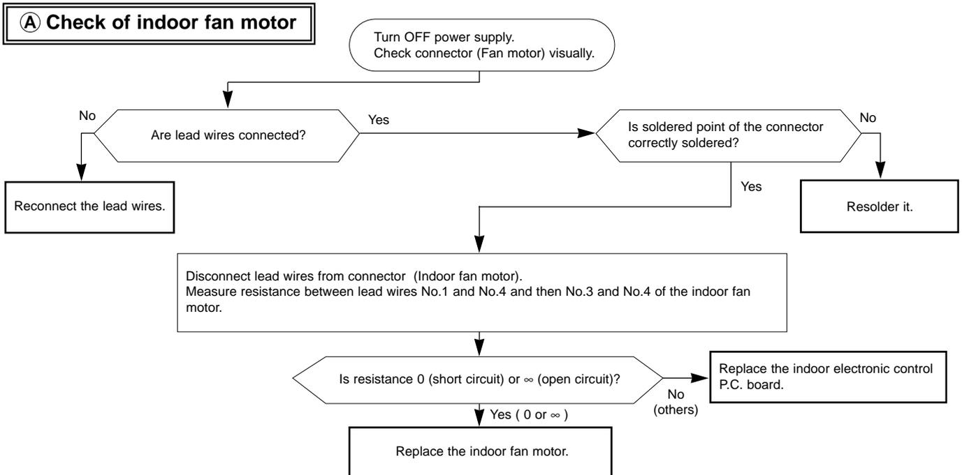
Indoor unit operates by pressing the EMERGENCY OPERATION switch, but does not operate with the remote controller.
