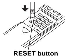
**NOTE:** 1. If RESET button is not pressed, the remote controller may not operate correctly.
