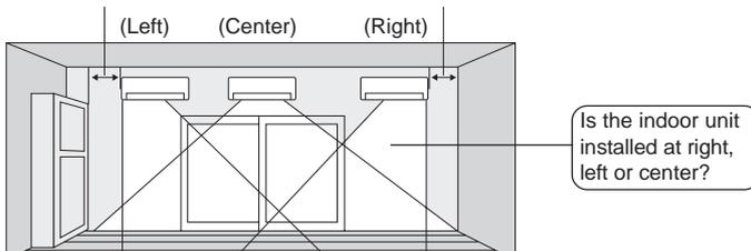
**NOTE:** If the indoor unit is installed more than 50 cm away from the side walls, cabinets or other nearby objects, set the slide switch to the "center" position.
