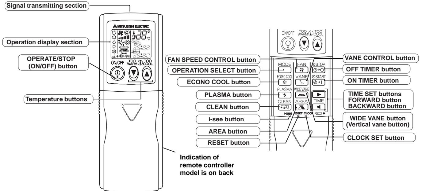
**NOTE:** Last setting will be stored after the unit is turned OFF with the remote controller. Indoor unit receives the signal of the remote controller with beeps.
