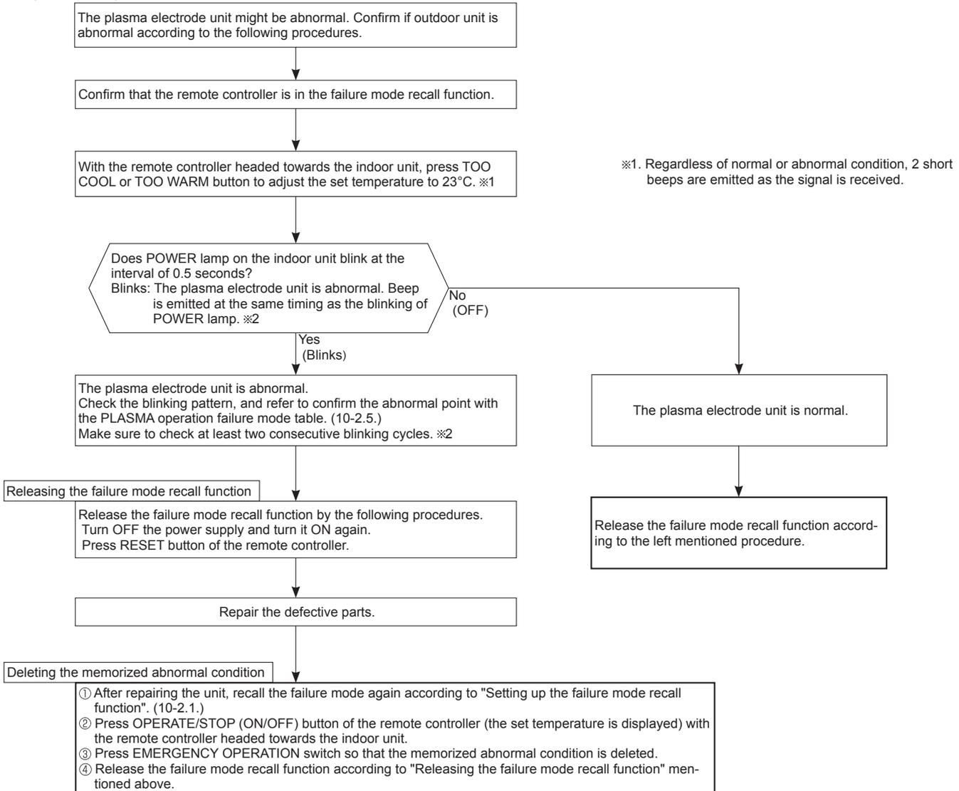
**NOTE:** 1. Make sure to release the failure mode recall function once it is set up, otherwise the unit cannot operate properly.
