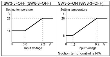
\*When the setting temperature in heating mode is  $17^{\circ}$ C or less, the discharge air temperature can be unstable.
