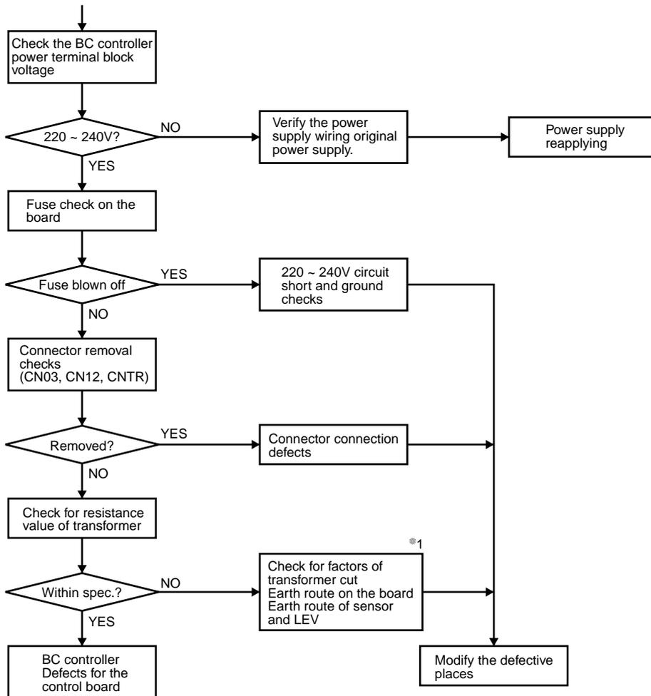
\*1 As for transformer checks, It is subject to the failure judgment method of main parts in 4.5.
