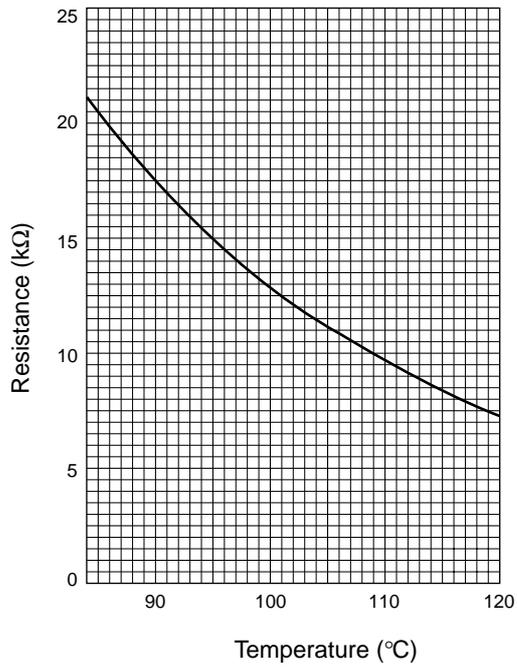
Thermistor  $R_0 = 33\text{k}\Omega \pm 1\%$  (TH2)
