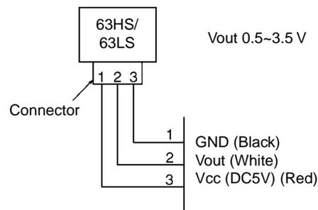
\* Connector connection specifications on the pressure sensor body side.
