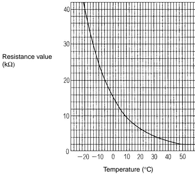
Thermistor  $R_0=15\text{ k}\Omega$
