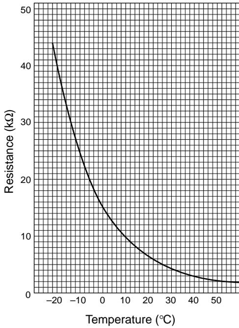
Thermistor  $R_{120} = 7.465\text{k}\Omega \pm 2\%$  (TH1, 10)
