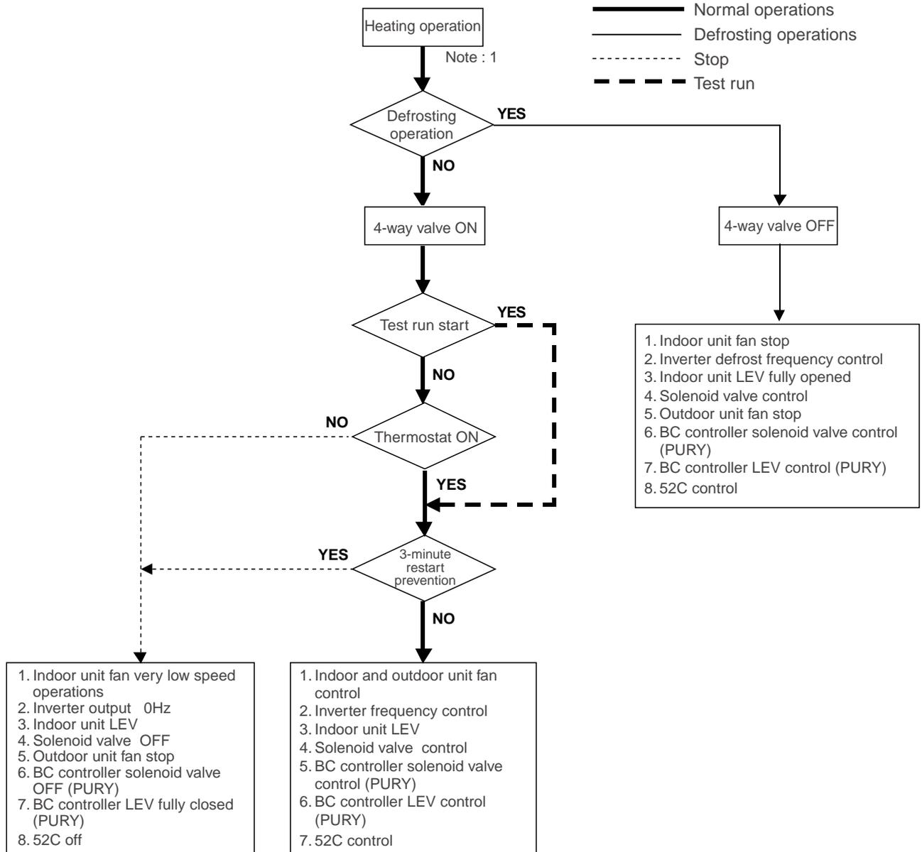
Note : 1 When outdoor unit starts defrosting, it transmits defrost operations command to (BC controller and) indoor unit, and the indoor unit starts defrosting operations. Similarly when defrosting operation stops, indoor unit returns to heating operation after receiving defrost end command of outdoor unit.
