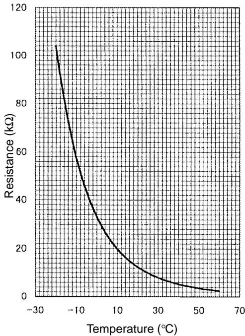
Thermistor  $R_{50} = 17\text{k}\Omega \pm 2\%$  (THHS)
