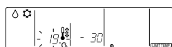
[When set temperature adjustment range in cool/dry mode is 19 °C to 30 °C]
