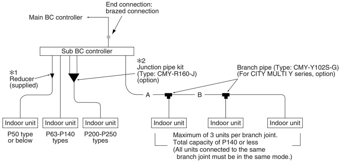
The size of the branch end connection on the BC controller is designed to fit P63-P140 type indoor units. To connect other types of indoor units, perform the following procedures.
