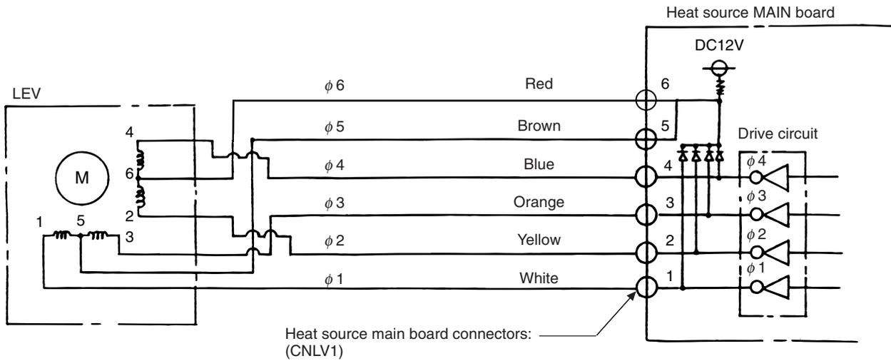
**Pulse signal output and valve operation**
