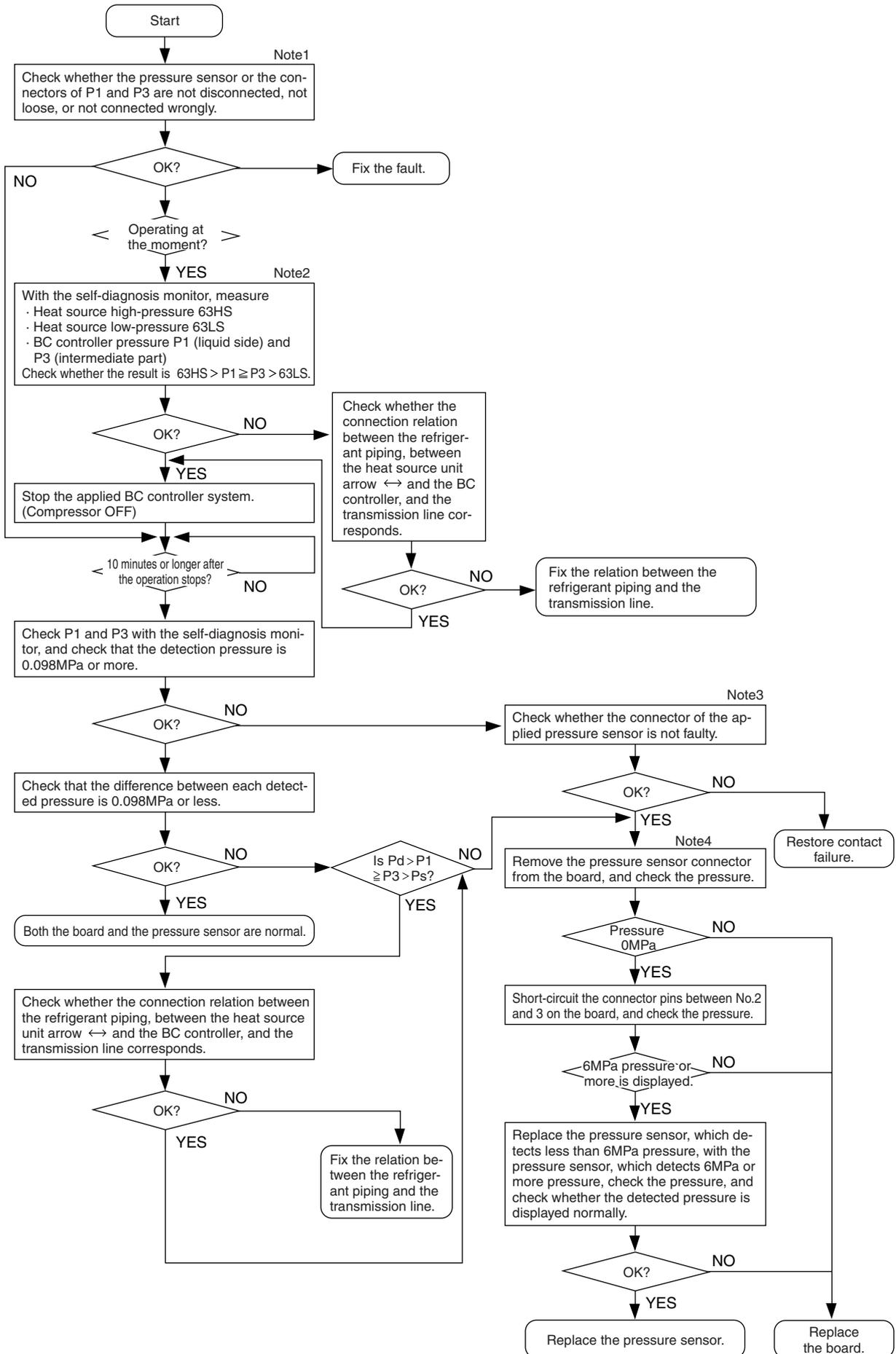
Note1 BC controller: Phenomena when the pressure sensor is connected wrongly (reverse connection of P1 and P3) to the board.
