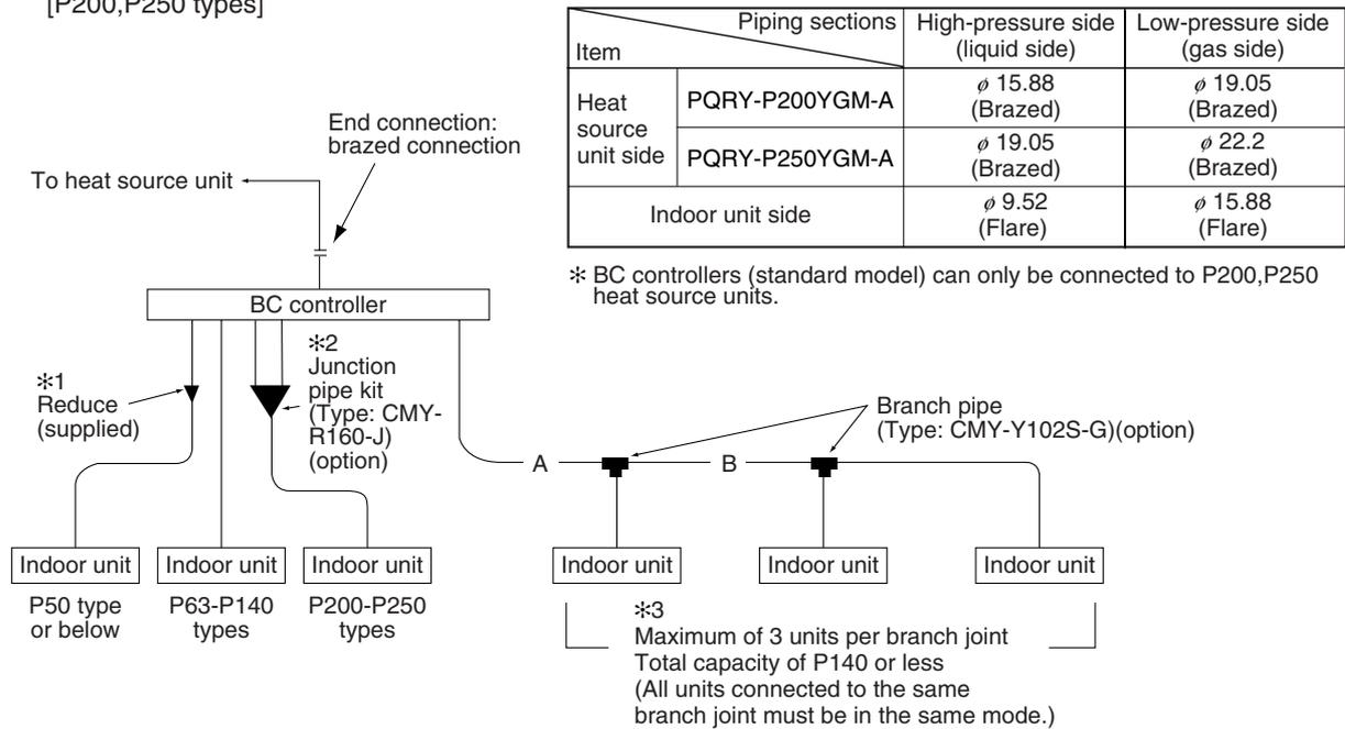
The size of the branch end connection on the BC controller is designed to fit P50-P140 type indoor units. To connect other types of indoor units, perform the following procedures.
