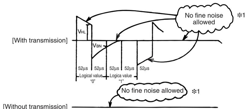
Check the wave shape of transmission line with an oscilloscope to confirm that the following conditions are being satisfied.
