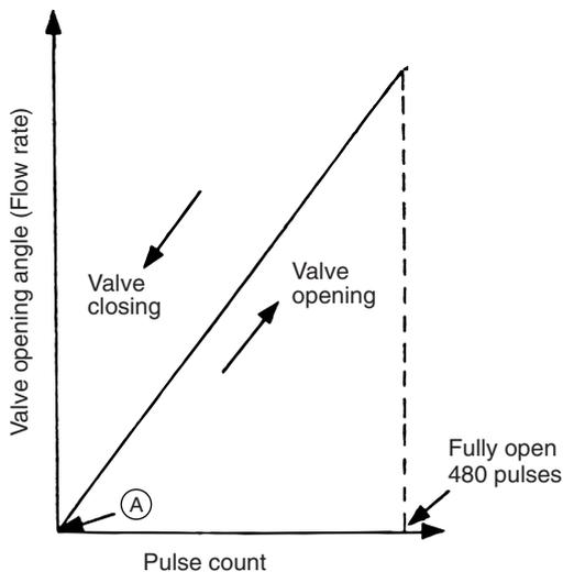
\* When the power is switched ON, a 520 pulse valve opening signal is output to make sure the valve's position, so that it is definitely at point (A). Pulse signal is output for approximately 17 seconds.
