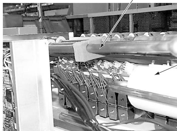
Tube-in-tube heat exchanger
