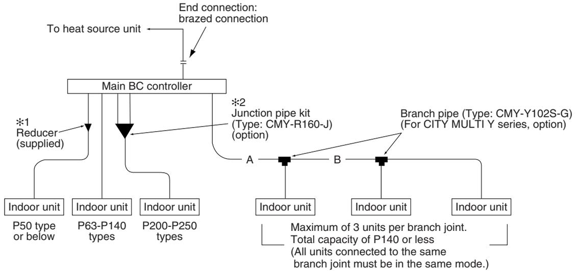
The size of the branch end connection on the BC controller is designed to fit P63-P140 type indoor units.
