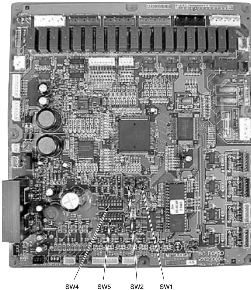
[ Relay board (RELAY 4 board) ]
