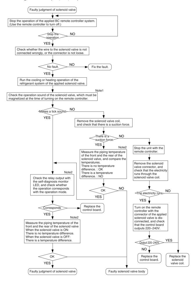
Check whether the BC board output signal and the solenoid valve operation correspond.
