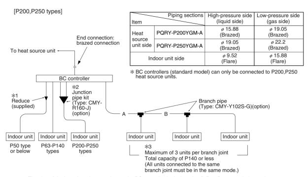
The size of the branch end connection on the BC controller is designed to fit P50-P140 type indoor units. To connect other types of indoor units, perform the following procedures.
