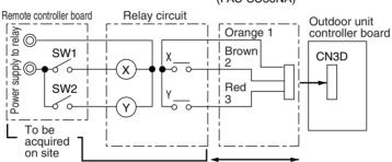
Maximum allowable length of wiring is 10 m.
