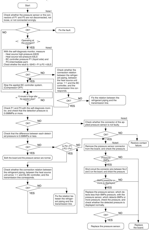
Note1 BC controller: Phenomena when the pressure sensor is connected wrongly (reverse connection of P1 and P3) to the board.
