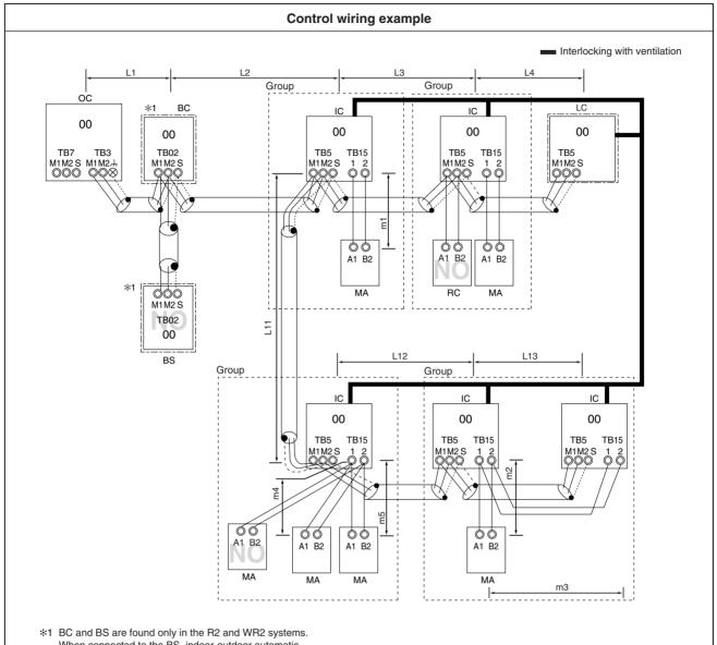
\*1 BC and BS are found only in the R2 and WR2 systems. When connected to the BS, indoor-outdoor automatic address start up function will not be available.
