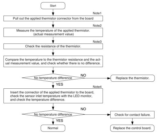
Note1 For the connectors on the board, TH11~TH12 is CN10, and TH15 and TH16 is CN11. Disconnect the applied connector, and check every number of the sensor.
