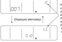
If registration is successfully completed, the two displays as shown on the left will appear alternately.
