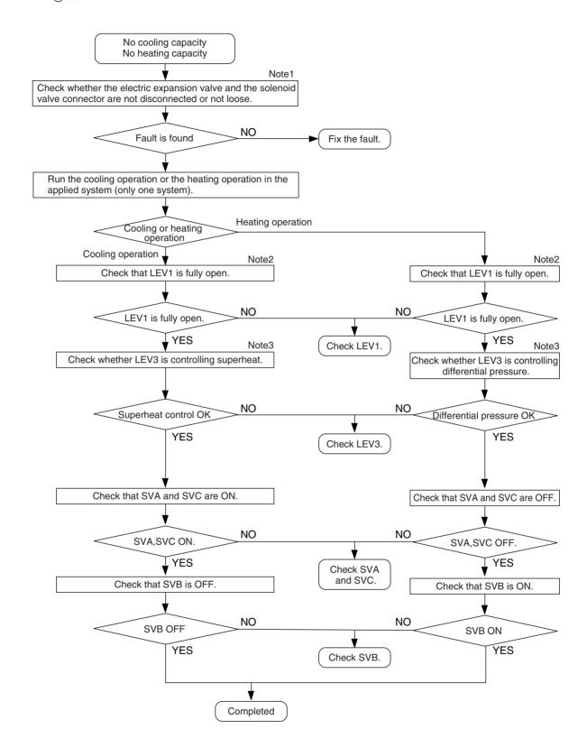
Note1 BC controller: Phenomena when LEV is connected wrongly (reverse connection of LEV1 and LEV3) to the board.
