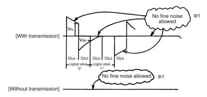
Check the wave shape of transmission line with an oscilloscope to confirm that the following conditions are being satisfied.
