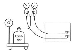
For a cylinder without a syphon attached
