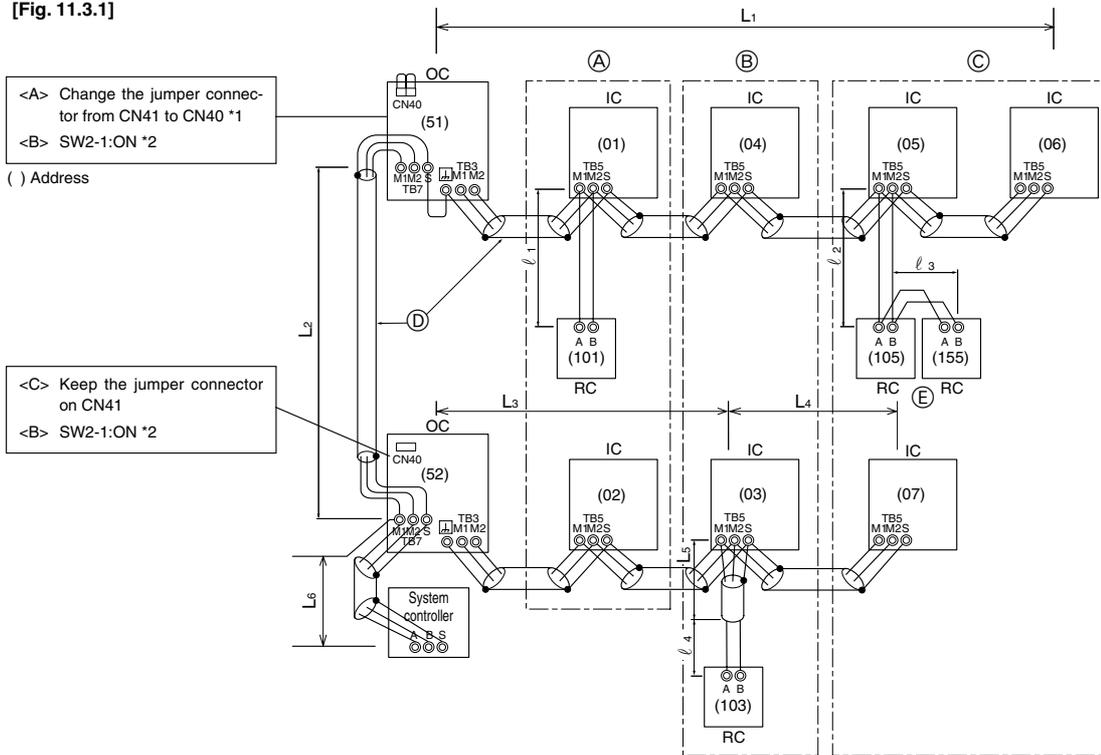
\*1: When the power supply unit is not connected to the transmission line for centralized control, disconnect the male power supply connector (CN41) from ONE outdoor unit in the system and connect it to CN40.
