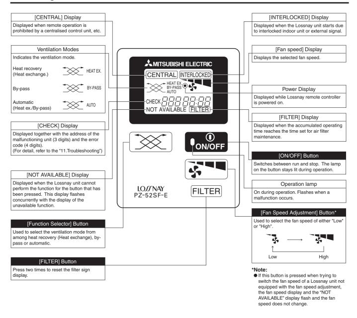
This remote controller can not be used on Lossnay units set for interlocked operation with Mr. Slim units.
