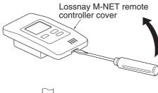
4. Remove the Lossnay M-NET remote controller cover using a standard screw-driver. Attach the Lossnay M-NET remote controller unit to the switch box using the two enclosed cross-recessed pan head screws. Use a standard screwdriver with a blade that is 4 mm or wider to remove the cover.
