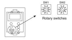
Set the Lossnay M-NET remote controller address.
