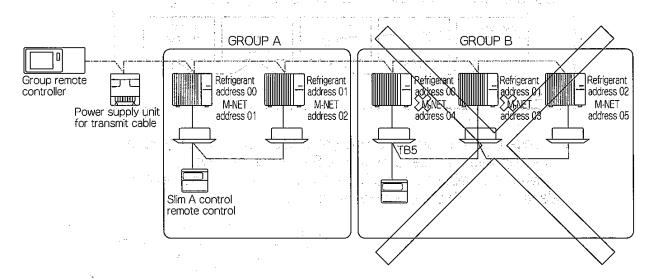
\*It is not good with the above setting in the group B because the outdoor unit which has the refrigerant address 00 does not have the minimum M-NET address 3 in the group. Make the outdoor unit of the refrigerant address set with the minimum address in the group like the group A.
