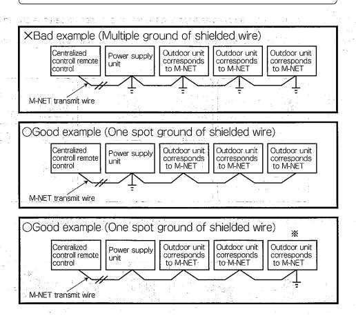
\*In case that the outdoor unit is grounded, connect the ground wire supplied as accessory to the S terminal (secondary) of M-NET terminal bed and M-NET Ground terminal inside of electric box with using screws supplied.
