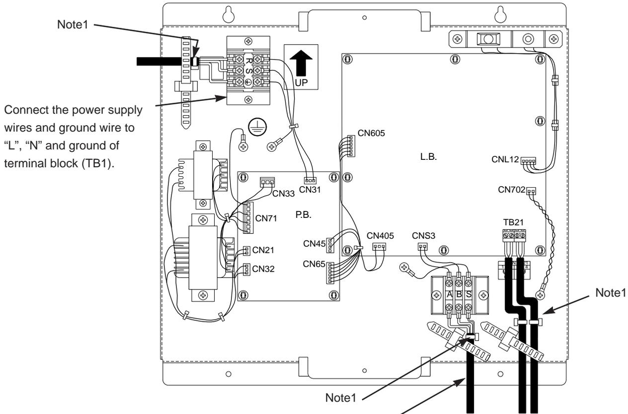
Connect the power supply wires and ground wire to "L", "N" and ground of terminal block (TB1).
