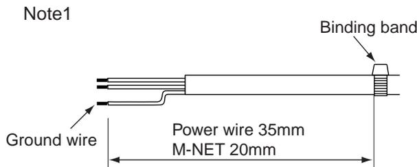
For power wire and M-NET transmission wire
