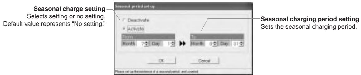
Figure 8-5 TG-2000A seasonal charge setting screen (ex, electric power manual input, pulse count)
