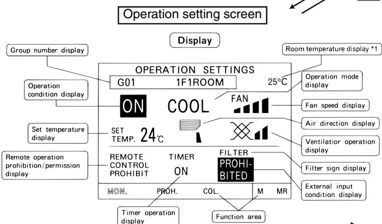
\*The following settings are possible using the Operation Panel switches
