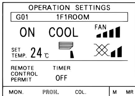
① Press the switch to display the group that the operation prohibition setting will be performed.
