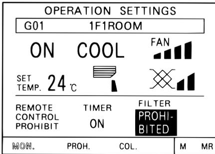
The **PROHIBITED** is displayed and the prohibition operation is display in reverse display when operation of this controller is prohibited by another system controller or an external input signal used. The prohibition operation which is displayed in reverse display is not possible to operate in this condition.
