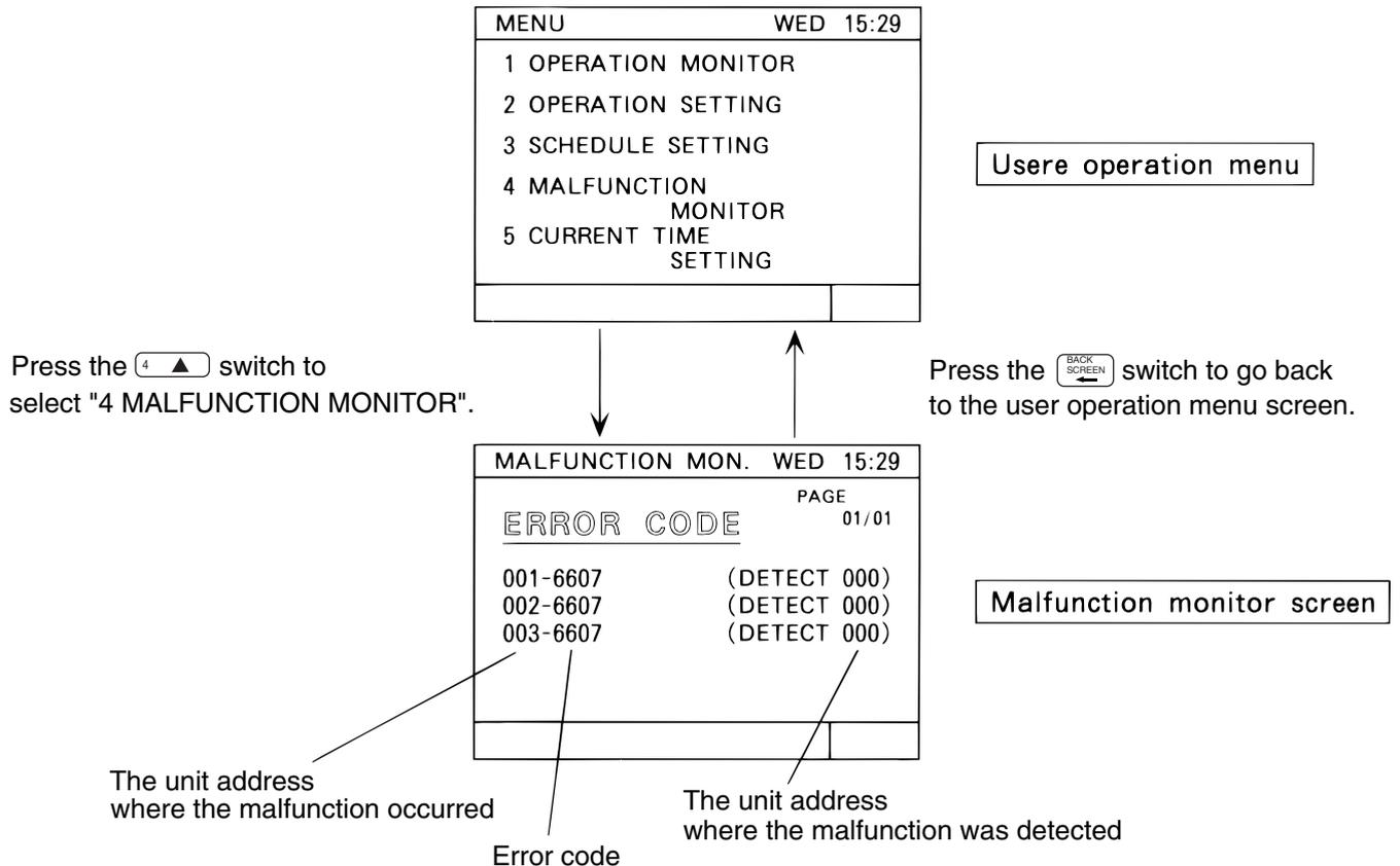
**NOTE :** When there is no malfunction taking place, [ NO ERROR ] lights up instead of [ ERROR CODE ].
