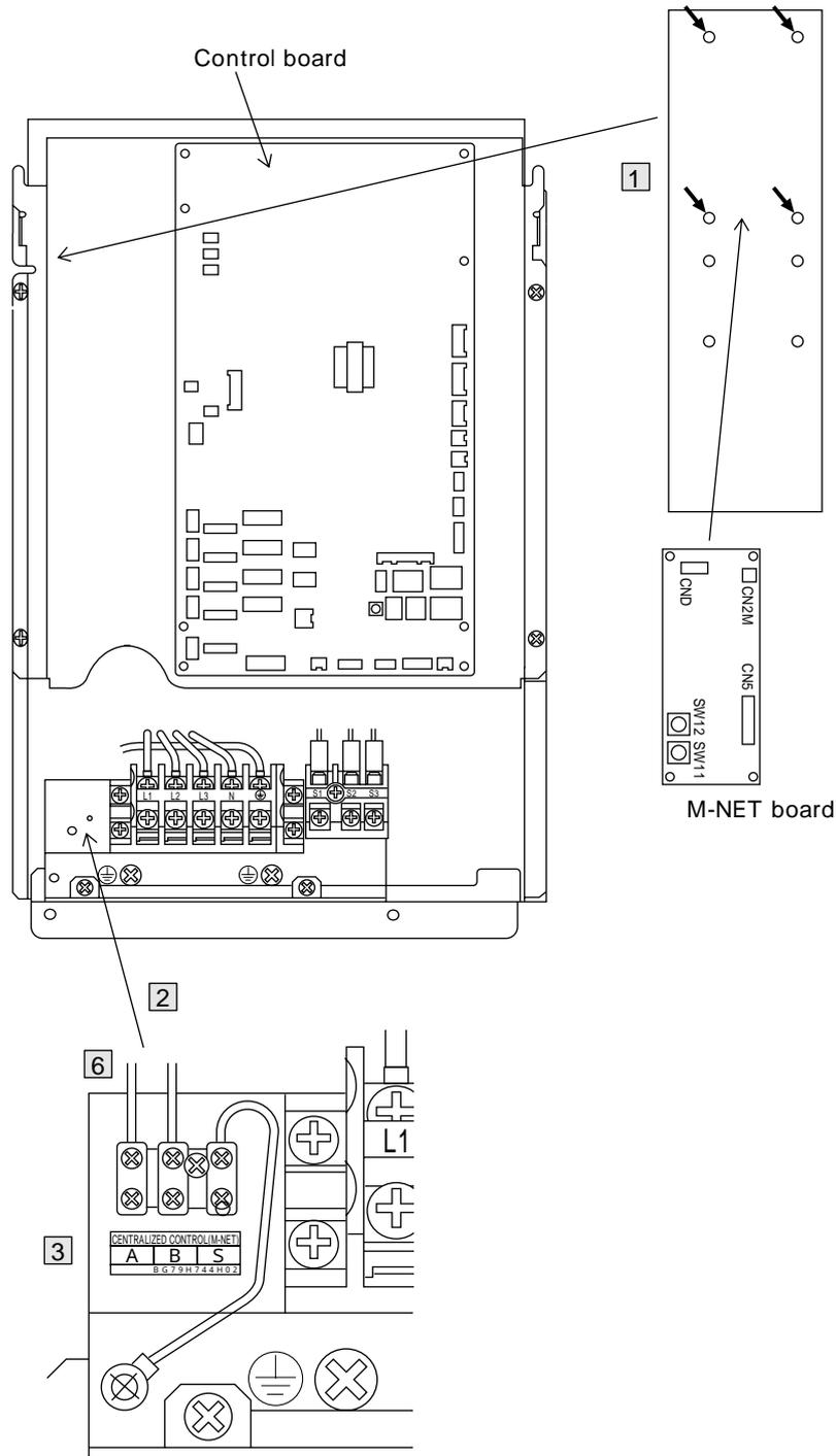
**1** Install M-NET board (with insulation sheets and supports) on the side of electric box .
