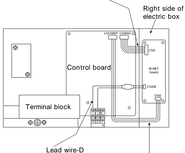
7 Connection of M-NET board (CN2M) and Terminal block (Terminals A & B)
