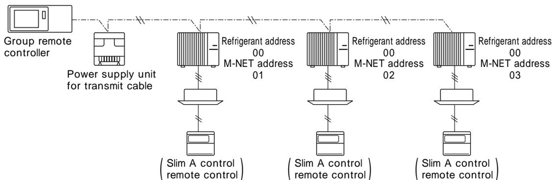
Between the outdoor units, it is OK that only M-NET wiring (2 wires, no polarity) is done.
