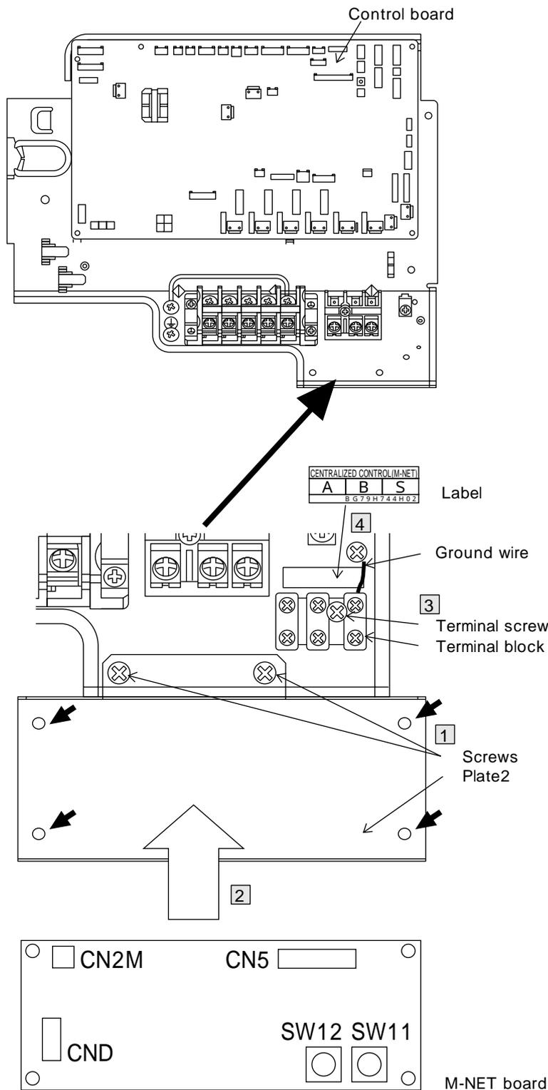
1 Attach the Plate 2 , using two screws .
