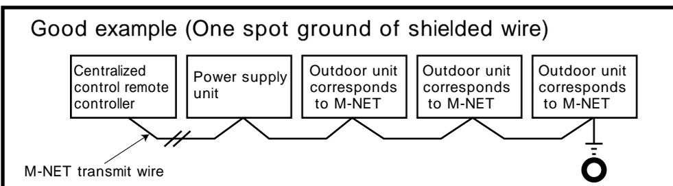
In case that the outdoor unit is grounded, connect the ground wire supplied as accessory to the S terminal (secondary) of M-NET terminal block and M-NET Ground terminal inside of electric box with using screws supplied.
