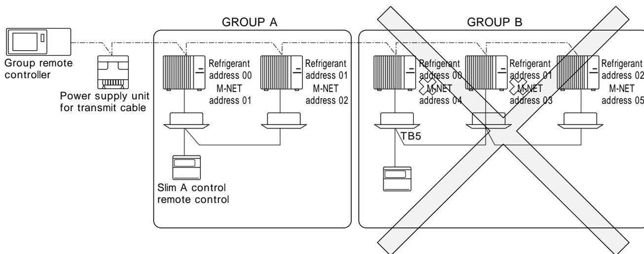
It is not good with the above setting in the group B because the outdoor unit which has the refrigerant address 00 does not have the minimum M-NET address 3 in the group. Make the outdoor unit of the refrigerant address set with the minimum address in the group like the group A.
