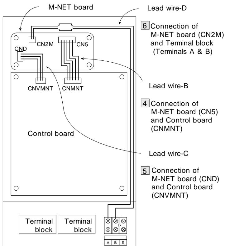
1 Install the M-NET board so that the (SW11, SW12) come front.
