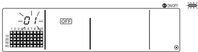
● When system startup communication is completed, □ the Group Setting/Monitor Screen will open.
