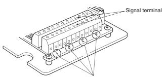
\* Connect the devices corresponding to their display number on the control panel.
