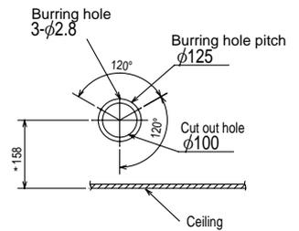
( Connected the attached flexible pipe or socket. )
