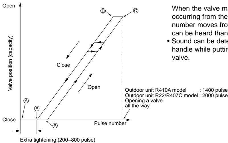
When the valve moves smoothly, there is no sound or vibration occurring from the linear expansion valves; however, when the pulse number moves from ⑤ to ④ or when the valve is locked, more sound can be heard than in a normal situation.
