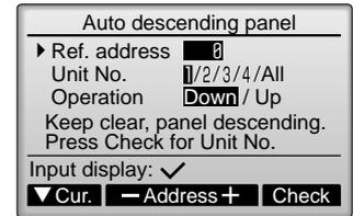
Select the refrigerant address and the unit number for the units to whose falls panel, with the **F2** or **F3** button, and press the button.
