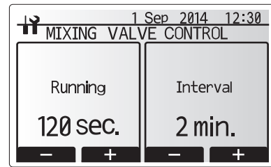
Mixing valve control setting screen
