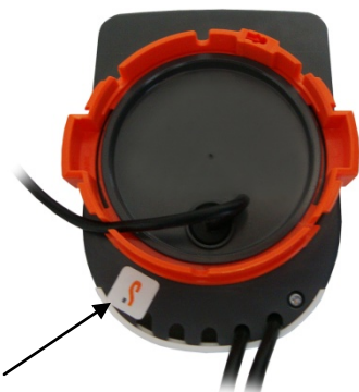
Seal installed in the factory on the integrator
