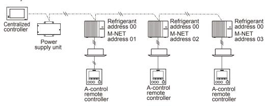
It is acceptable if M-NET wire (non-polar, 2-cores) is arranged in addition to the wiring for A-control.
