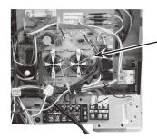
Noise filter circuit board (N.F.)
