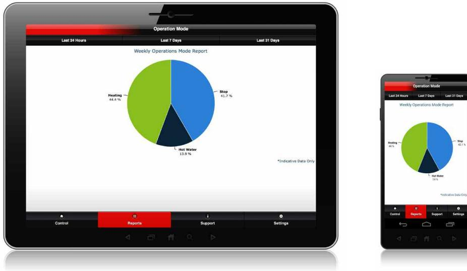
The Operation Mode Report provides a way to view indicative\* percentages of time the Mitsubishi Electric Ecodan Heating system has been in specific operation state. The Operation Mode Reports can provide a view of recent and historical operational information which could be useful when analysing usage patterns.
