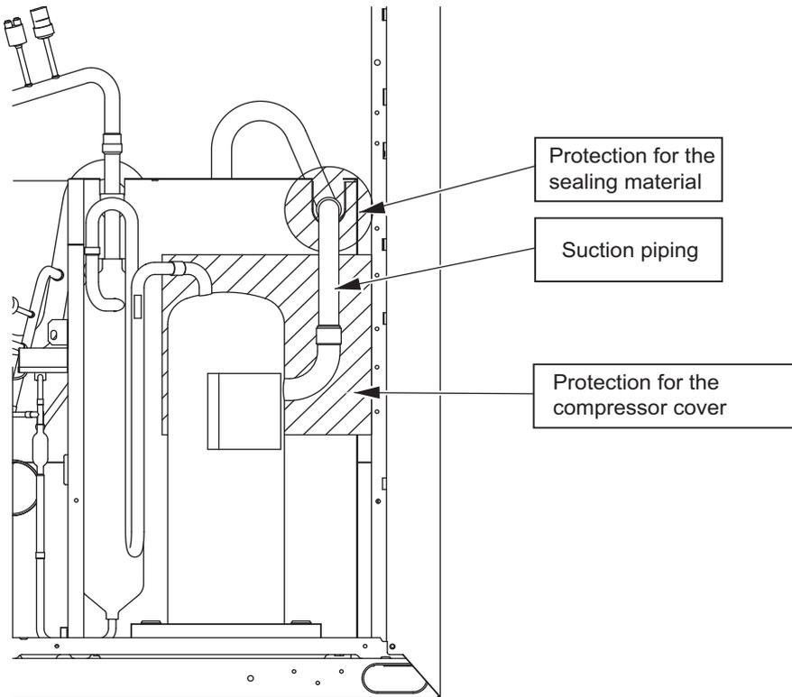
6. Place protective materials on the insulation lining of the compressor cover and on the sealing material on the compressor suction pipe to protect them from the torch flame, debraze the pipe, and replace the compressor.
