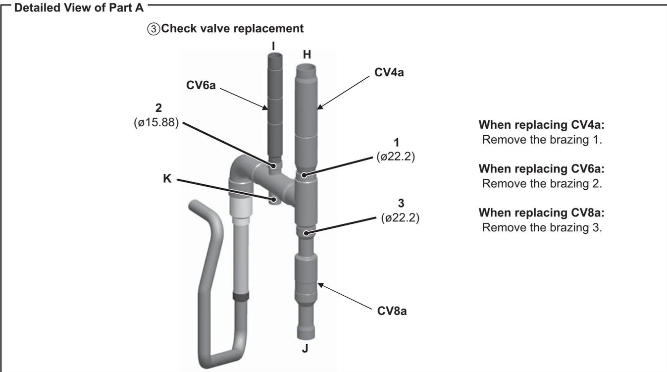
**R410A CITY MULTI R2 Solenoid valve block ASSY (SV4a, SV4b, SV4d), Check valve (CV4a, CV6a, CV8a, CV9a) replacement instructions**
