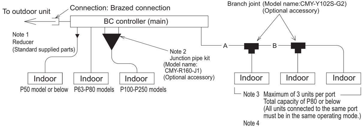
Note 4 Group the indoor units together that connected to the same port if multiple indoor units are connected to the same port on BC controller. Also share one thermo-stat such as on remote controller so that they turn on/off at the same time.
