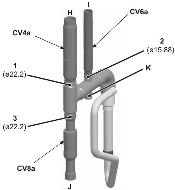
**When replacing CV4a:**
