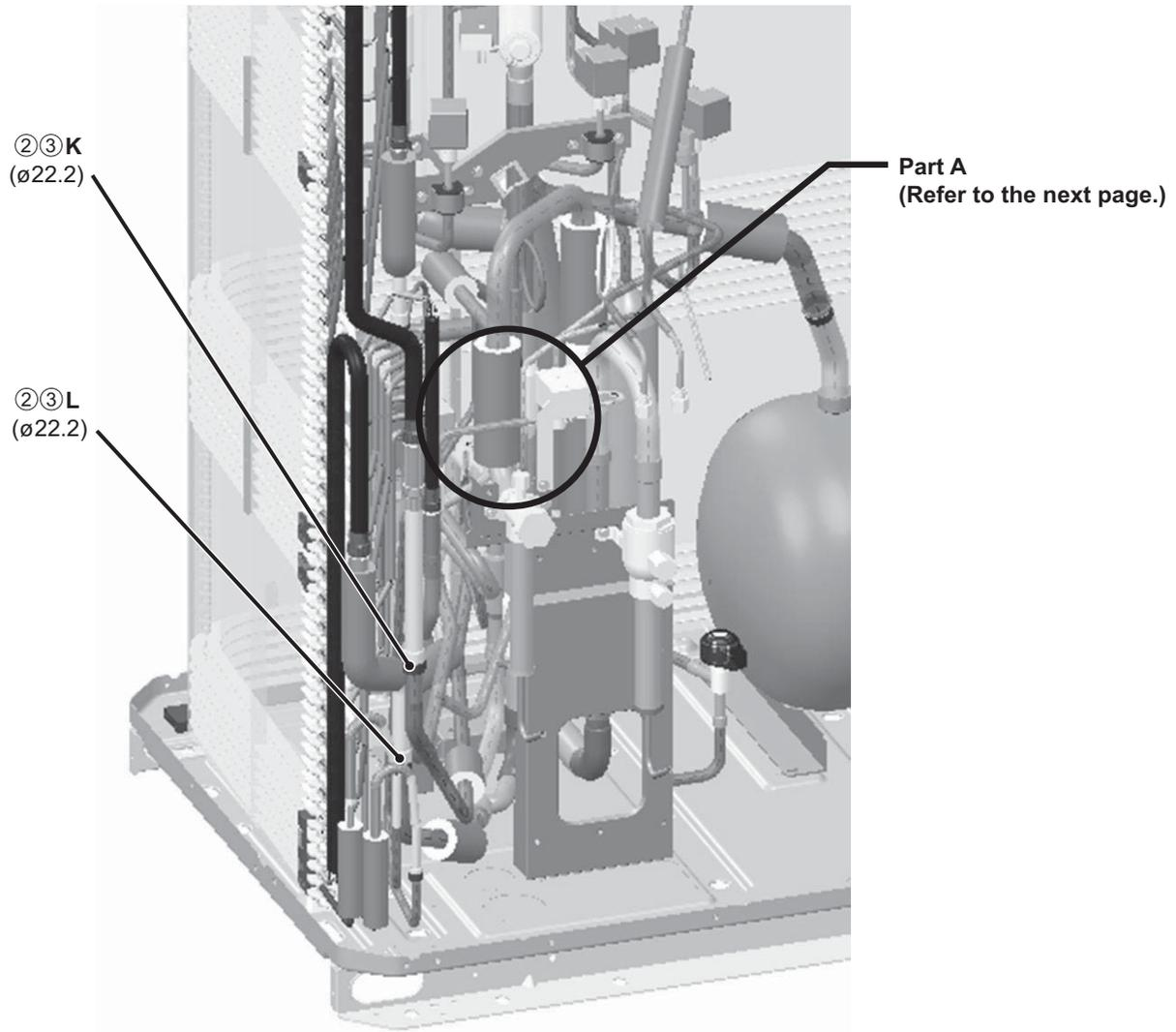
\* After removing Solenoid valve block ASSY
