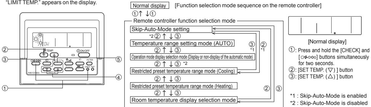
[6-4 Selecting Remote Controller Functions from an ME Remote Controller ]
