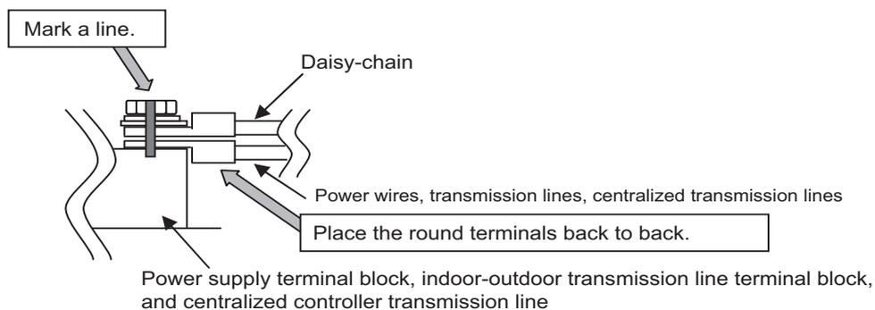
Poor contact caused by loose screws may result in overheating and fire.
