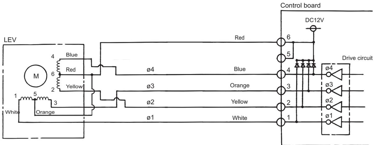
3) Pulse signal output and valve operation
