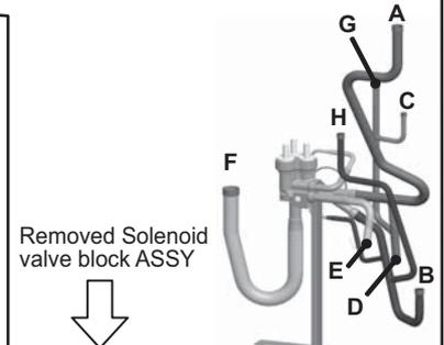
⑤⑥ Removing or fixing the Supporting plate for Solenoid valve block
