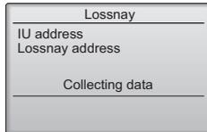
[2] When the search is completed, the smallest address of the indoor units that are connected to the remote controller and the address of the interlocked LOSSNAY unit will appear. "--" will appear if no LOSSNAY unit is interlocked with the indoor units.
