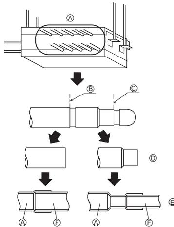
Be sure to have pipe expansion of indoor unit connecting port by cutting the piping at the cutting point which depends on the indoor unit capacity.
