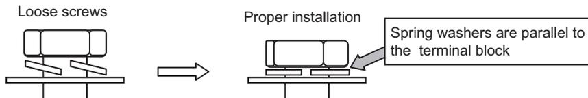
2) Check the wires are securely fastened to the screw terminals.
