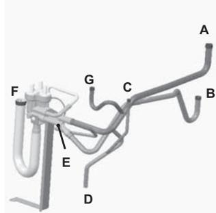
Removed Solenoid valve block ASSY
