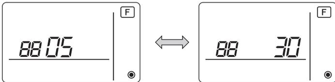
Cannot be registered because the registered indoor unit or LOSSNAY does not exist.
