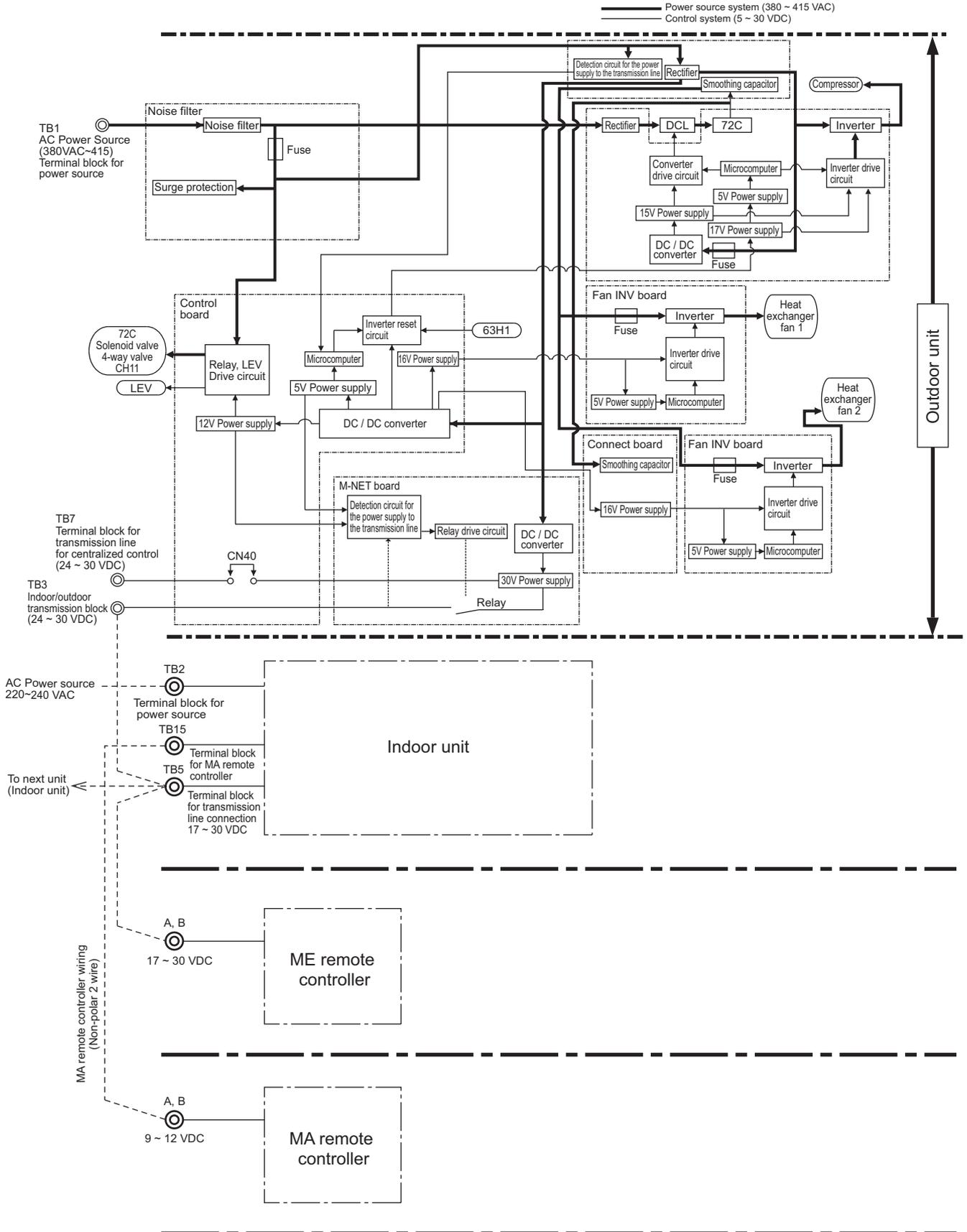
\* MA remote controllers and ME remote controllers cannot be used together.
