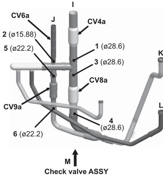
**When replacing CV4a:**
