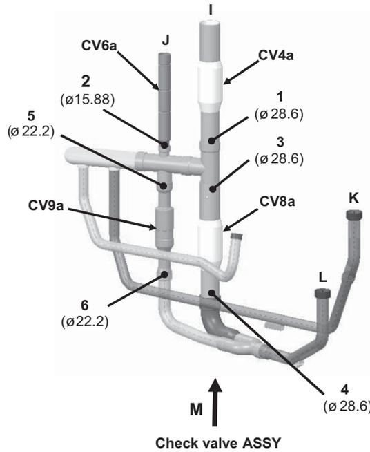
When replacing CV4a:
