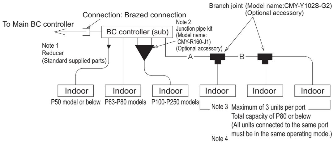
The ports of the BC controller accommodates the pipes on P63-P140 models of indoor units. To connect other types of indoor units, follow the procedure below.
