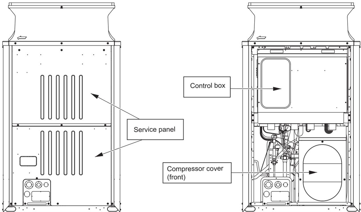
1. Remove both the top and bottom service panels (front panels).
