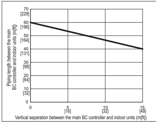
**(2) System that requires more than 16 BC controller ports or with multiple BC controllers <System with one outdoor unit>**
