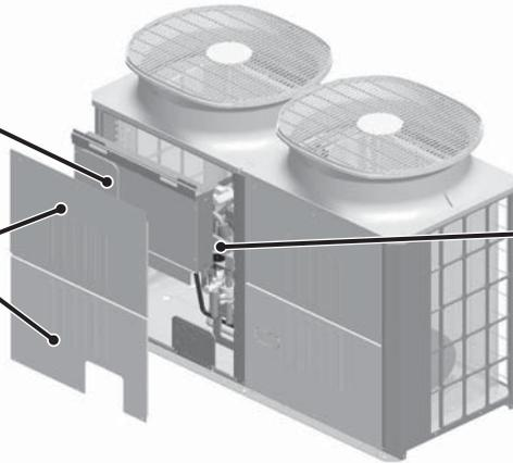
3) Remove the cable that is fixed to the Frame M ASSY and remove the Frame M ASSY.
