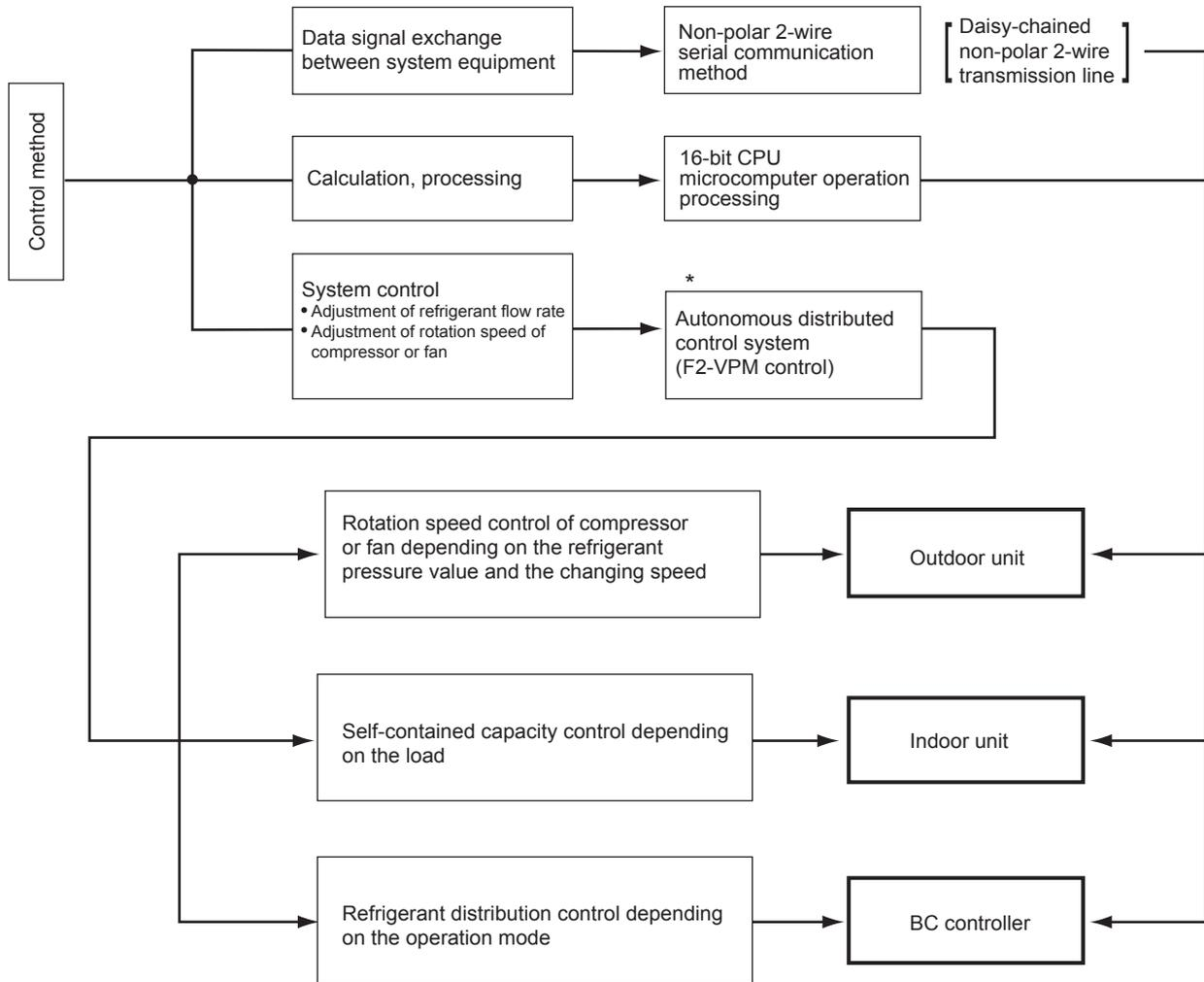
Autonomous distributed control system : A system that consists of three independent sub control systems, instead of a single centralized control system, that work together to maintain the overall control of the entire system.
