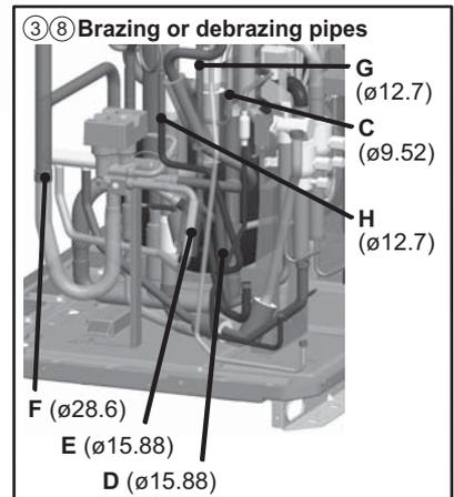
\*This figure does not show heat exchanger.
