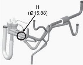
②⑧ Removing or installing solenoid valve block
