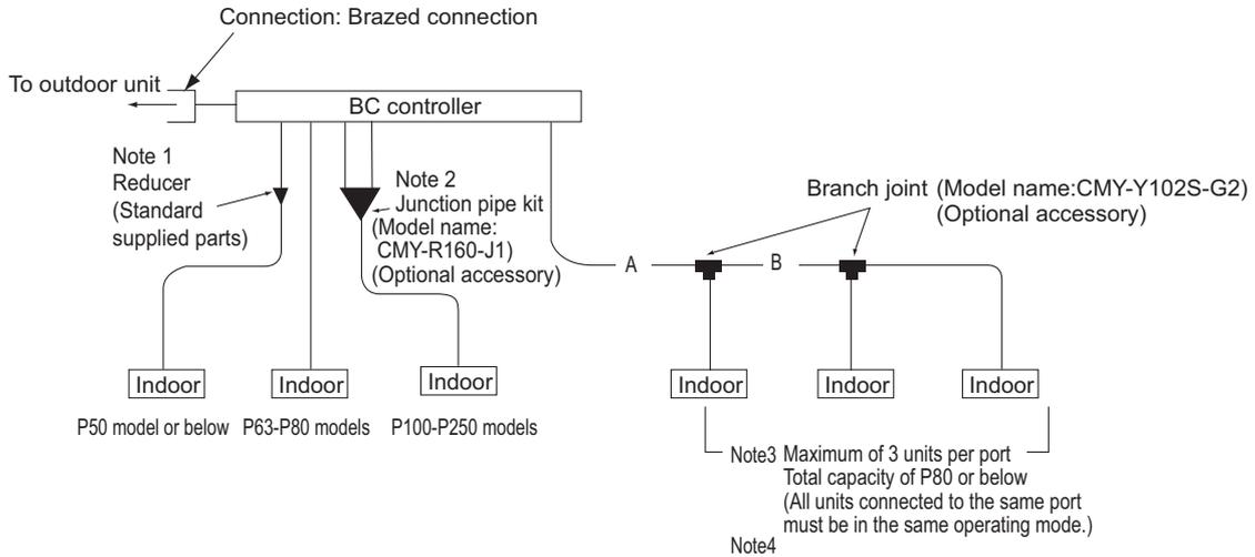
Note 4 Group the indoor units together that connected to the same port if multiple indoor units are connected to the same port on BC controller. Also share one thermo-stat such as on remote controller so that they turn on/off at the same time.
