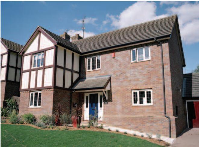
The Luton house has a total area of 177m<sup>2</sup>, with double glazed windows, loft insulation and cavity wall insulation. The previous heating system had been an 80% efficient gas boiler providing 23.2kW of heat from an input of 29kW. Existing radiators had a flow temperature of 70°C with a total output of 13.4kW. Hot water demand was 140 litres per day.
