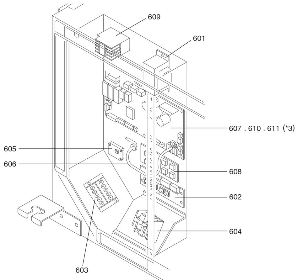
\*3 Parts No. 607 cannot be used with the indoor units with a production number of 06W\*\*\*\*\* or later.
