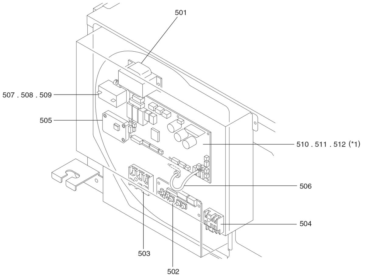
\*1 Parts No. 510 cannot be used with the indoor units with a production number of 06W\*\*\*\*\* or later.
