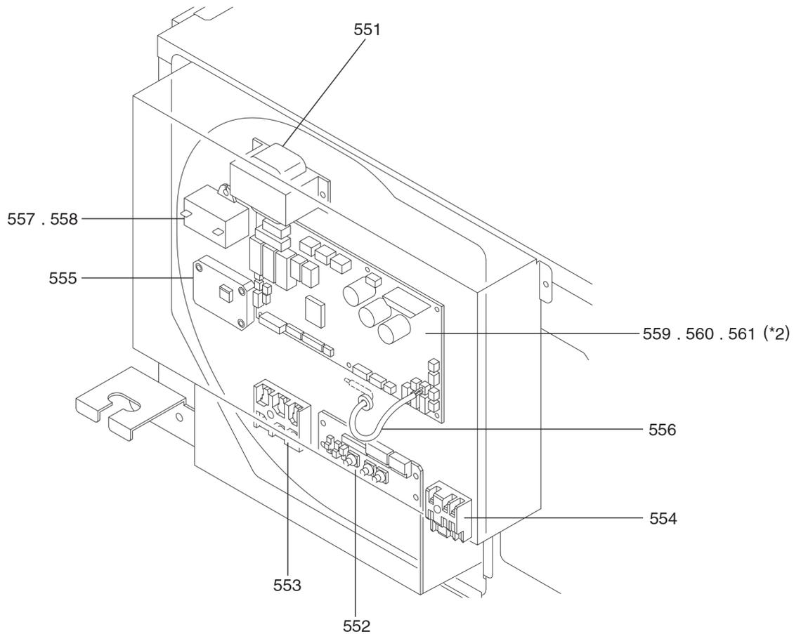
\*2 Parts No. 559 cannot be used with the indoor units with a production number of 06W\*\*\*\*\* or later.
