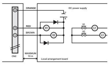
Note: 24v DC power supply and relays required for run and fault outputs.
