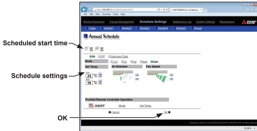
Set the start time to apply to the schedule, set the operations to be scheduled, and then press [OK]. The operations that can be scheduled for air conditioning unit groups are as follows: ON/OFF/Optimized Start, Mode, Set Temp, Air Direction, Fan Speed, and Prohibit Remote Controller Operation.
