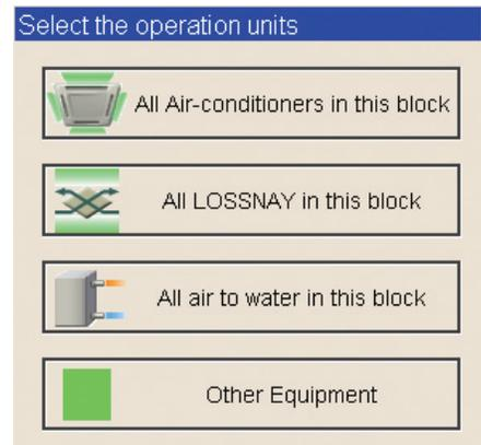
The 'Select the operation units' dialog box has a blue title bar and four buttons with icons: 'All Air-conditioners in this block', 'All LOSSNAY in this block', 'All air to water in this block', and 'Other Equipment'.
