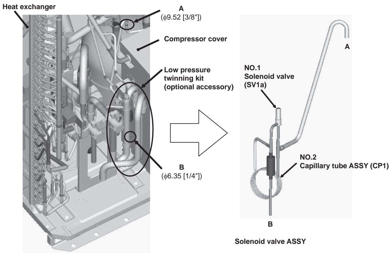
① Debraze A and B, and remove solenoid valve ASSY from the unit.
