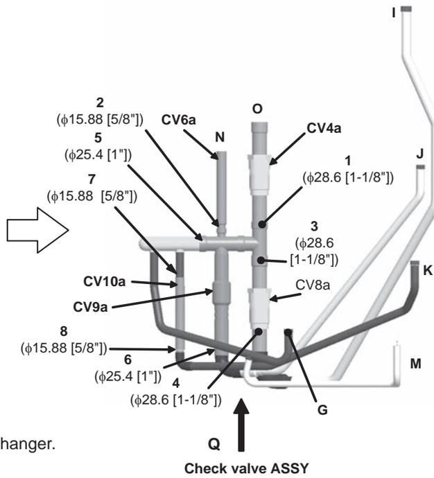
**When replacing CV4a:**
