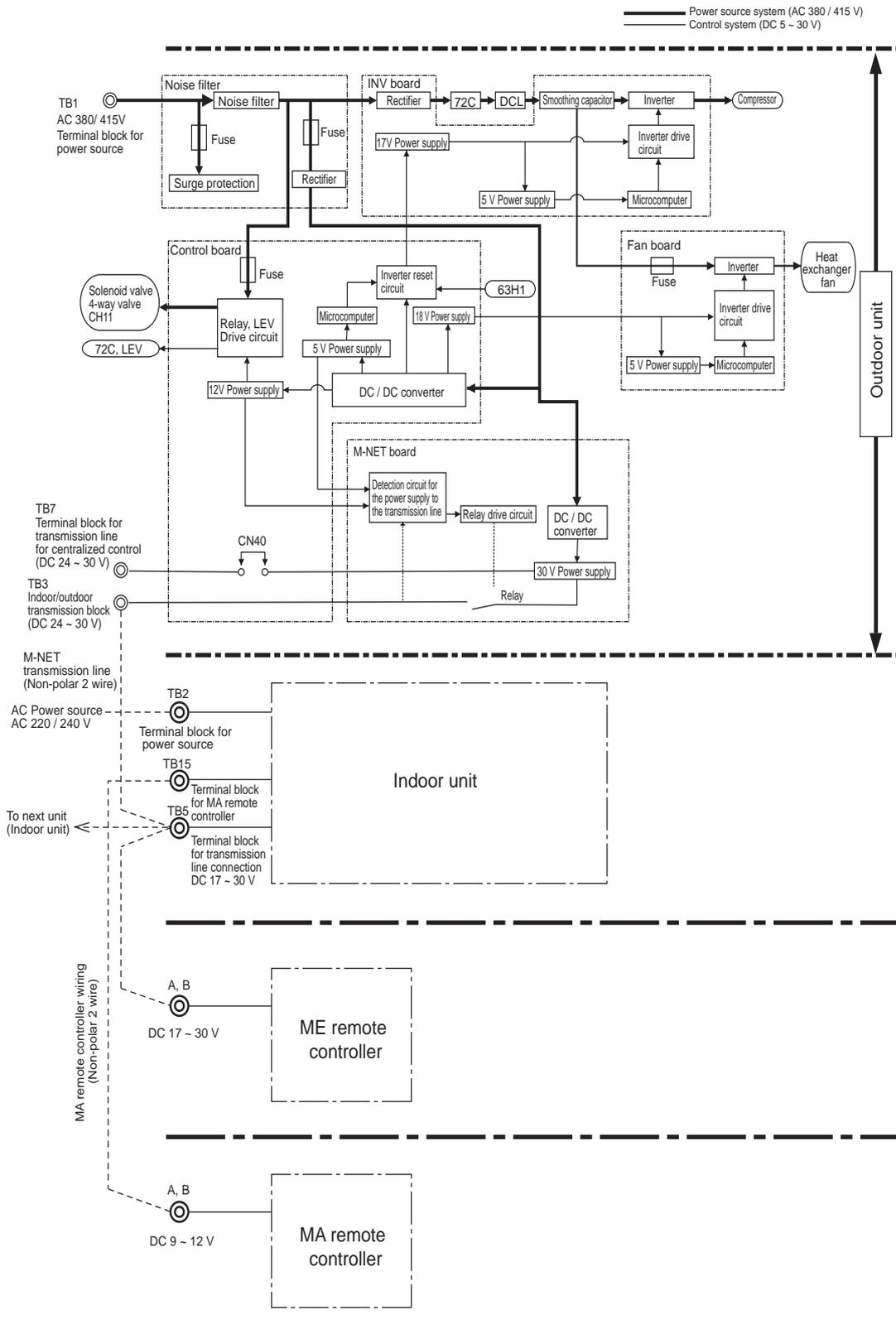
\* MA remote controllers and ME remote controllers cannot be used together.
