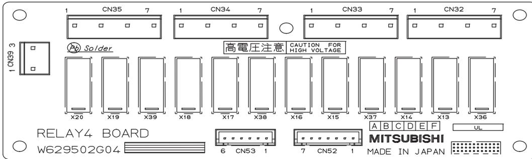
3. RELAY BOARD (RELAY 10 board)
