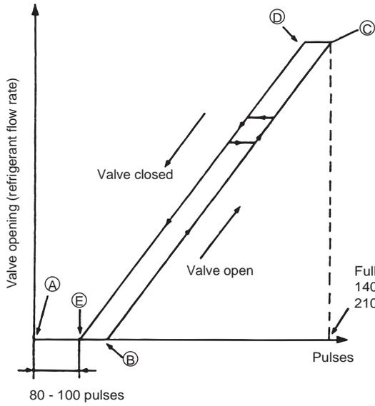
\*When the power is turned on, the valve closing signal of 2200 pulses (Indoor LEV, BC controller LEV1 (G1 type only), and LEV3), or 3200 pulses (BC controller LEV1 (GA1 type only)), will be output from the indoor board to LEV to fix the valve position. It must be fixed at point **A**
