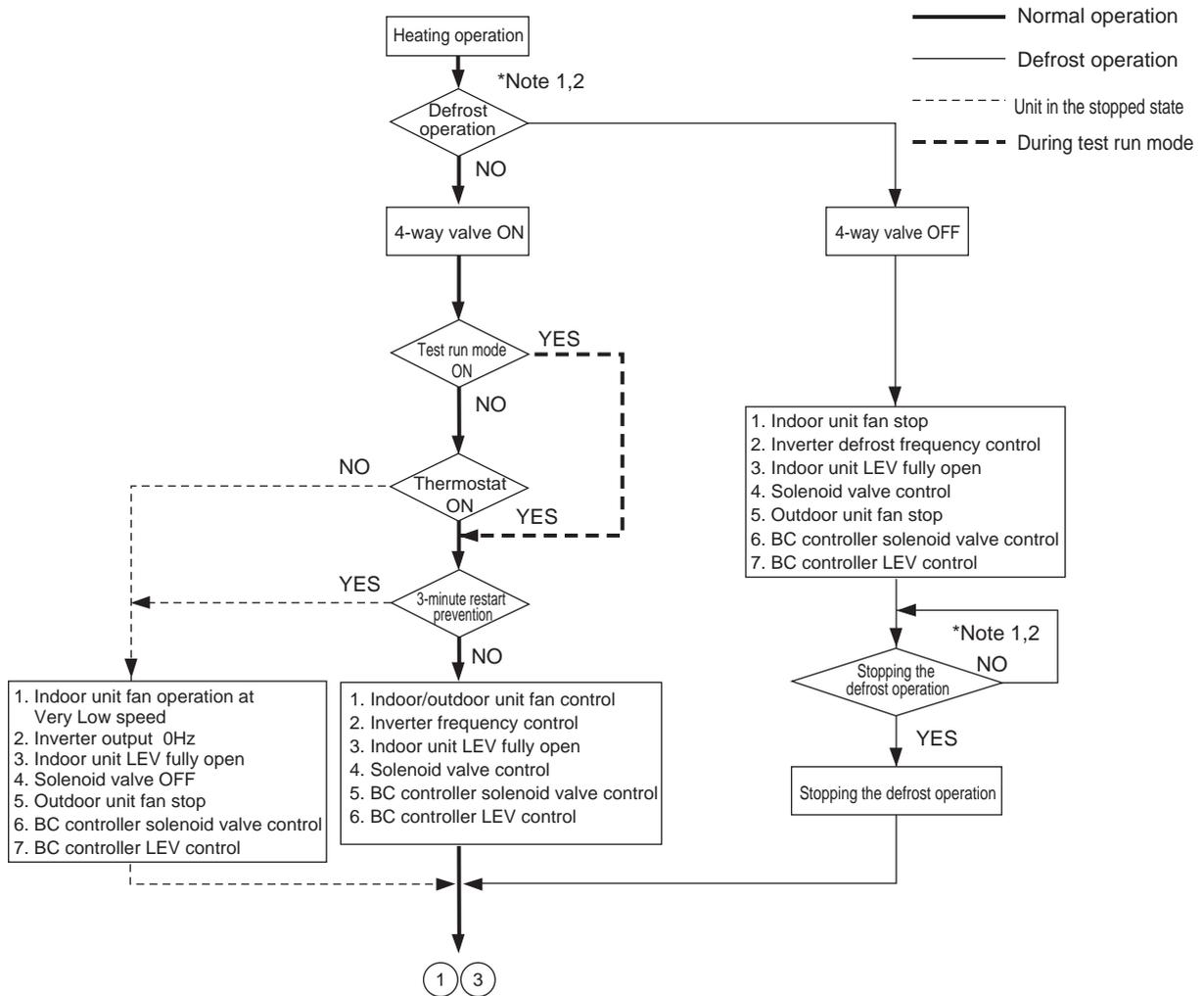
\*Note 1. When the outdoor unit goes into the defrost mode, defrost command is sent to the BC controller and indoor units. Upon reception of the command, the indoor units will go into the defrost mode. When defrosting is completed and upon receiving the signal that indicates the completion of defrosting, indoor units will resume the heating operation.
