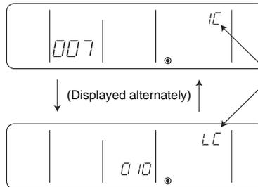
If registration is successfully completed, the two displays as shown on the left will appear alternately.
