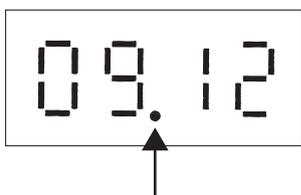
\* Disappears if the time data is deviated due to a power failure, or if a system controller that sets the time is not connected.
