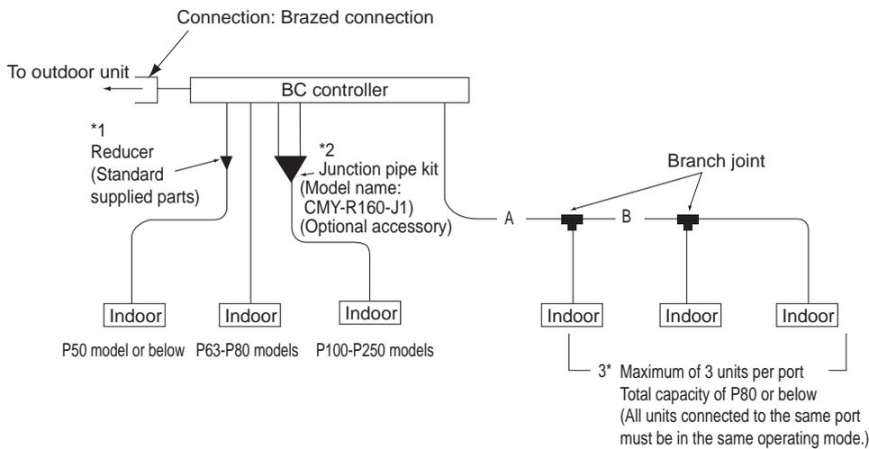
The ports of the BC controller accommodates the pipes on P63-P140 models of indoor units. To connect other types of indoor units, follow the procedure below.
