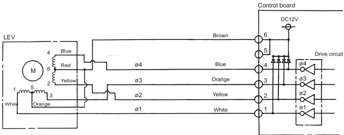
3) Pulse signal output and valve operation
