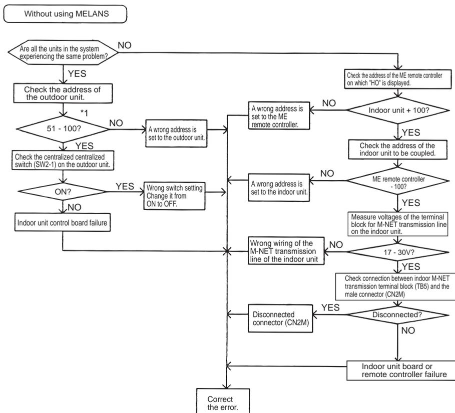
\*1. When the indoor unit address is set to 1 - 50, the address will be forcibly set to 100.
