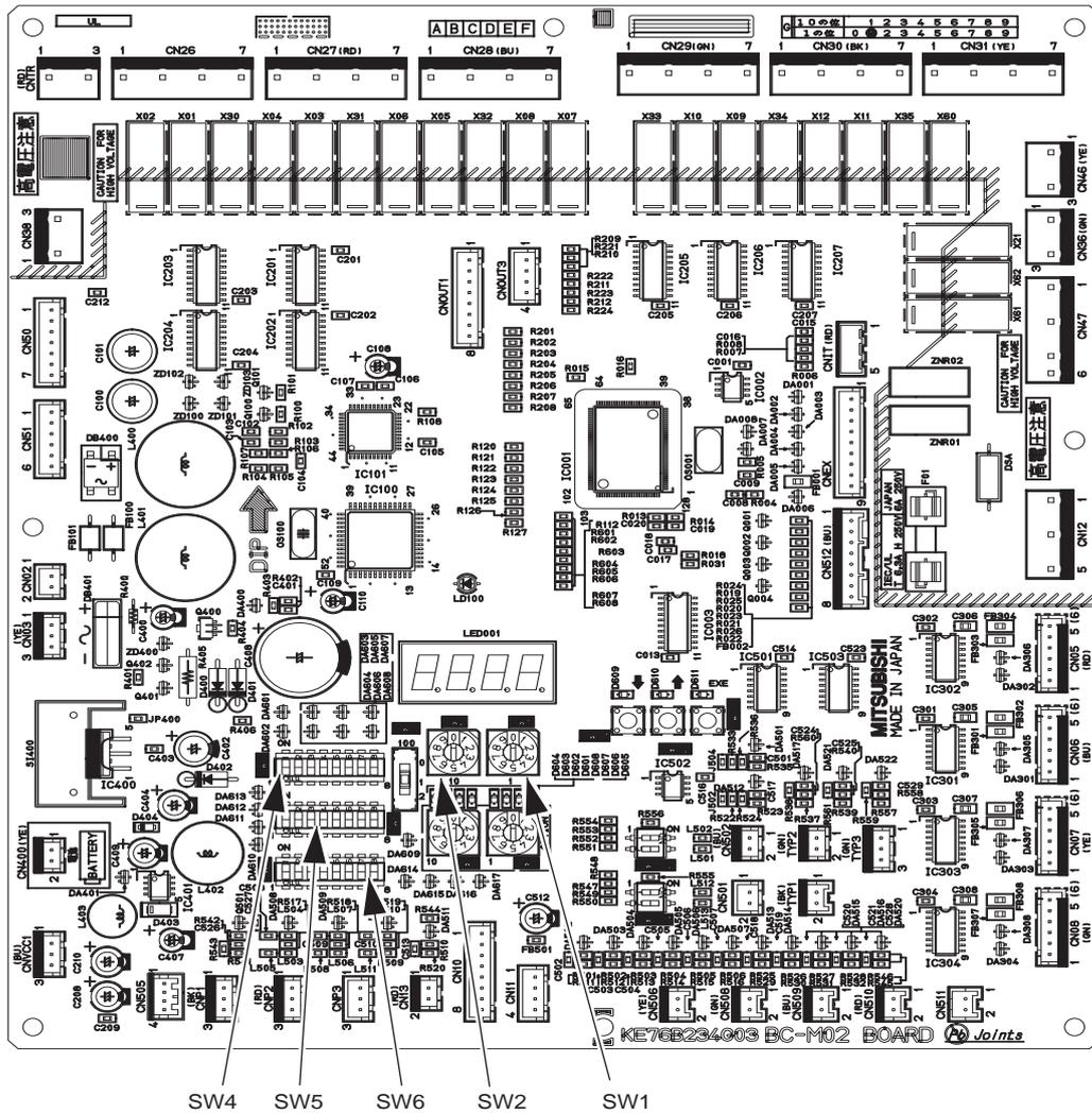
2. RELAY BOARD (RELAY 4 board)
