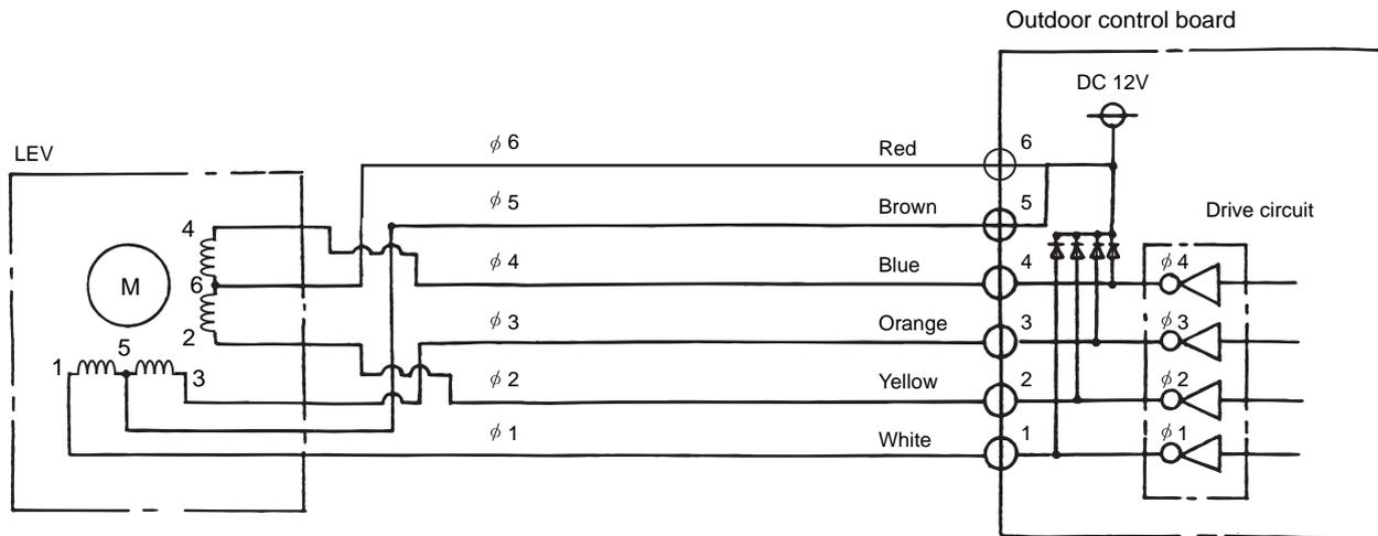
2) Pulse signal output and valve operation
