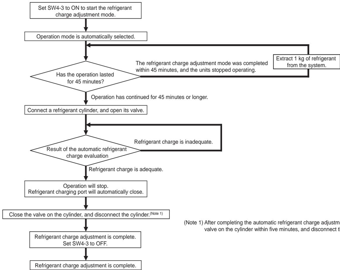
(Note 1) After completing the automatic refrigerant charge adjustment, close the valve on the cylinder within five minutes, and disconnect the cylinder.
