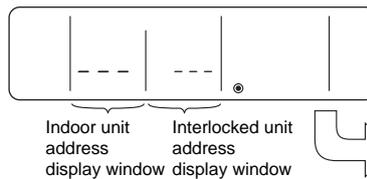
Both the “indoor unit address” and “interlocked unit address” will be displayed together.
