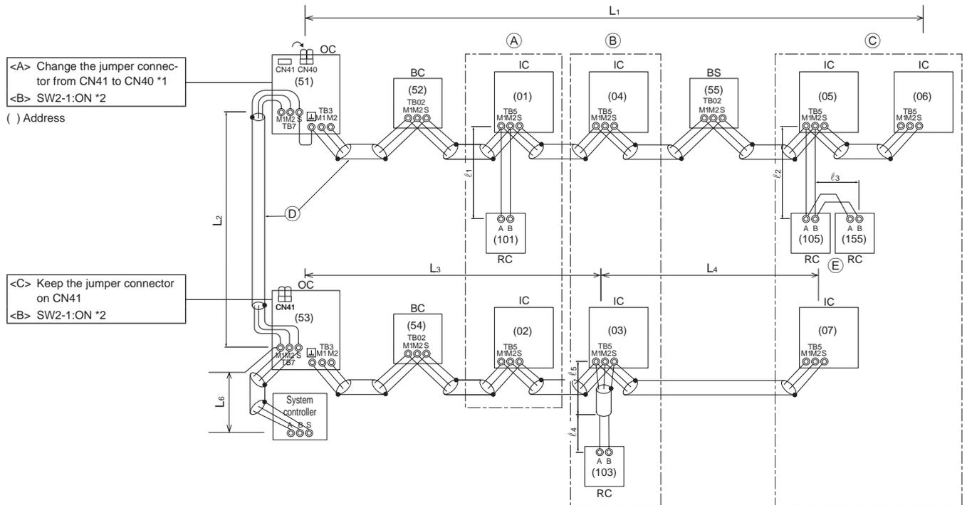
\*1 When the power supply unit is not connected to the transmission line for centralized control, disconnect the male power supply connector (CN41) from ONE outdoor unit in the system and connect it to CN40.
