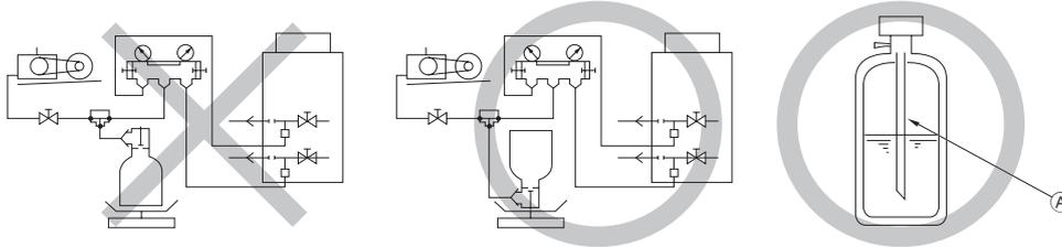
ⓑ: In case of the R410A cylinder having no syphon pipe.
