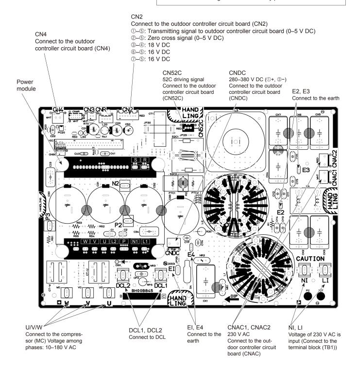
Outdoor power circuit board PUHZ-ZRP100YKA2.UK PUHZ-ZRP125YKA2.UK PUHZ-ZRP140YKA2.UK PUHZ-ZRP200YKA.UK PUHZ-ZRP250YKA.UK
