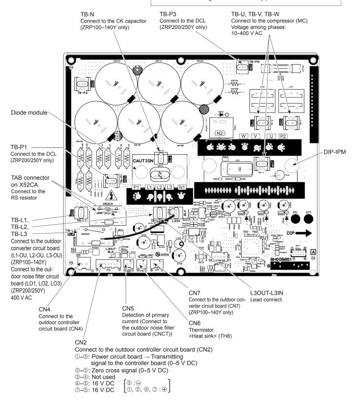
Outdoor converter circuit board PUHZ-ZRP100YKA2.UK PUHZ-ZRP125YKA2.UK PUHZ-ZRP140YKA2.UK
