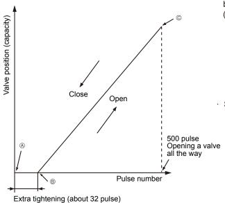
When the valve moves smoothly, there is no sound or vibration occurring from the linear expansion valve : however, when the pulse number moves from 8 to 6 or when the valve is locked, more sound can be heard.
