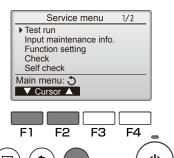
② Select "Test run" with the F1 or F2 button, and press the 🔾 button.
