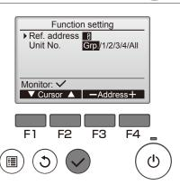
③ When data collection from the indoor units is completed, the current setting of the system appears highlighted.
