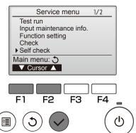
2 With the  $\fbox{F1}$  or  $\fbox{F2}$  button, enter the refrigerant address, and press the  $\textcircled{\checkmark}$  button.
