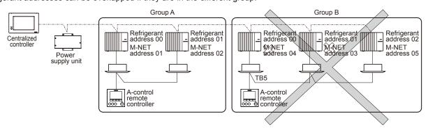
Note: In group B, M-NET address of the outdoor unit whose refrigerant address is "00" is not set to the minimum in the group. As "3" is right for this situation, the setting is wrong. Taking group A as a good sample, set the minimum M-NET address in the group for the outdoor unit whose refrigerant address is "00".
