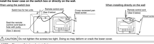
NOTE: • Choose a flat plane for installation • Fasten the switch box at more than two places when installing directly on the wall.
