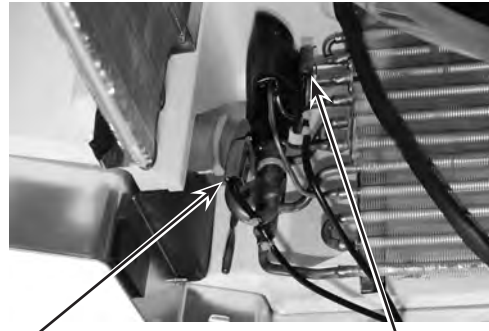
Condenser/evaporator temperature thermistor (TH5)
